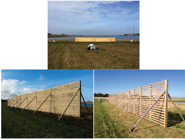
Figure 3. Photographs of the fence experiment. Top panel: overview of the fence and the instrumentation including the lidars and the mast. Left panel: solid and right panel: porous fence setups.
