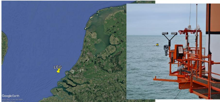
**Figure 1.** A map showing the location of the Lichteiland Goeree (LEG) platform, where concurrent rain and wind speed measurements were conducted (Caboni et al., 2024), and a picture of the OTT Parsivel<sup>2</sup> disdrometer installed on the platform are shown. Map courtesy of © Google Earth.
