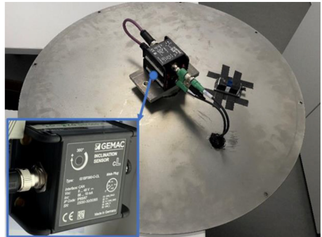
Figure 2. The 5 MN · m TTS manufactured by HBM (left image). It is a hollow-shaft transducer with flanges to be mounted in test benches. In the left image, the hollow shaft is covered by a cover plate. On the inside of this cover and placed centred is the inclinometer stack (zoom in right image). Moreover, a small sensor to log temperature and humidity inside the TTS is taped to the inner side of the cover plate (right image, black tape). Taken from Song et al. (2022).
