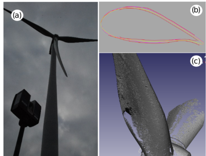
Figure 10. First blade scan operation: (a) 3D scanner on the ground close to the wind turbine, (b) scatter of possible blade sections that can be extracted from the cloud of points, and (c) missing data (“holes”) in the measured cloud of points from this first scan operation.
