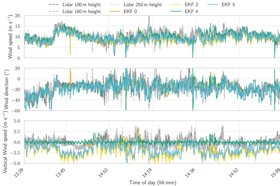
**Figure 21.** Test flight from 5 June 2024. Time series comparison of wind estimates from different EKF configurations, including a minimal sensor setup and three variants with additional inputs, against lidar observations. The plots show horizontal and vertical wind velocity components, as well as horizontal wind direction. Lidar data are available at 1 s resolution and are shown at three heights representative of the kite’s flight envelope.
