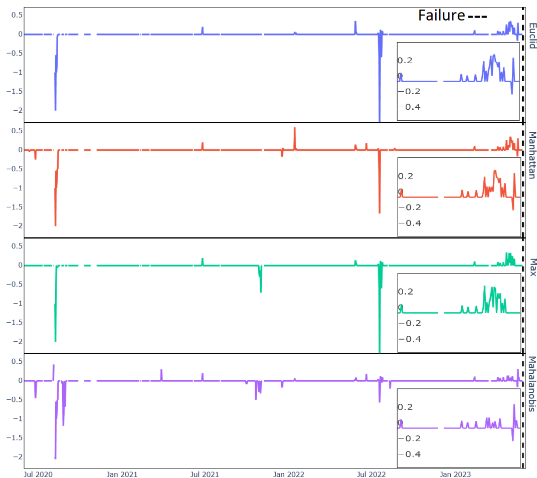
Figure 13. Filtered anomaly scores aggregated with a rolling average per day. The filtering was done with tuples constructed from all levels ( -3 to 3 ), using the Var95% threshold. The striped black line marks the start of the generator failure.
