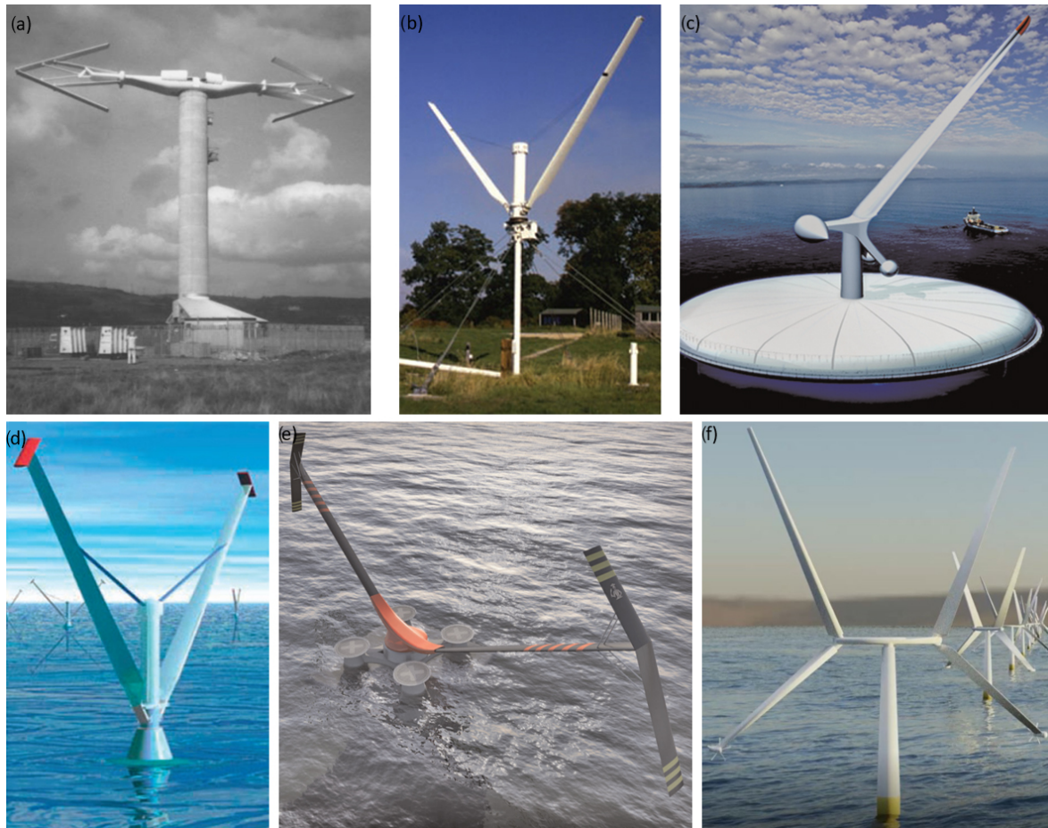
Figure 1. (a) Musgrove 250 turbine (Price, 2006), (b) 5 kW V-rotor tested by Sharpe and Derek Taylor (The Open University, 2015), (c) single-bladed V-rotor concept (Shires, 2013a), (d) Taylor V-turbine (The Open University, 2015), (e) the aerogenerator concept (Shires, 2013a), and (f) the X-rotor wind turbine concept.
