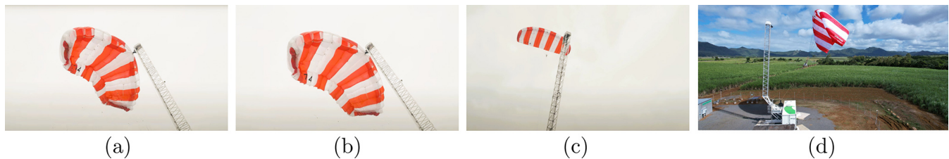
Figure 2. Principle of launching for a soft-wing kite AWES from SkySails Power GmbH (2024) during launch. (a) Deflated kite, (b) inflating kite, (c) airborne kite, and (d) overview of the system. Photos from SkySails Group (2024) and Sánchez-Arriaga et al. (2024, p. 47).
