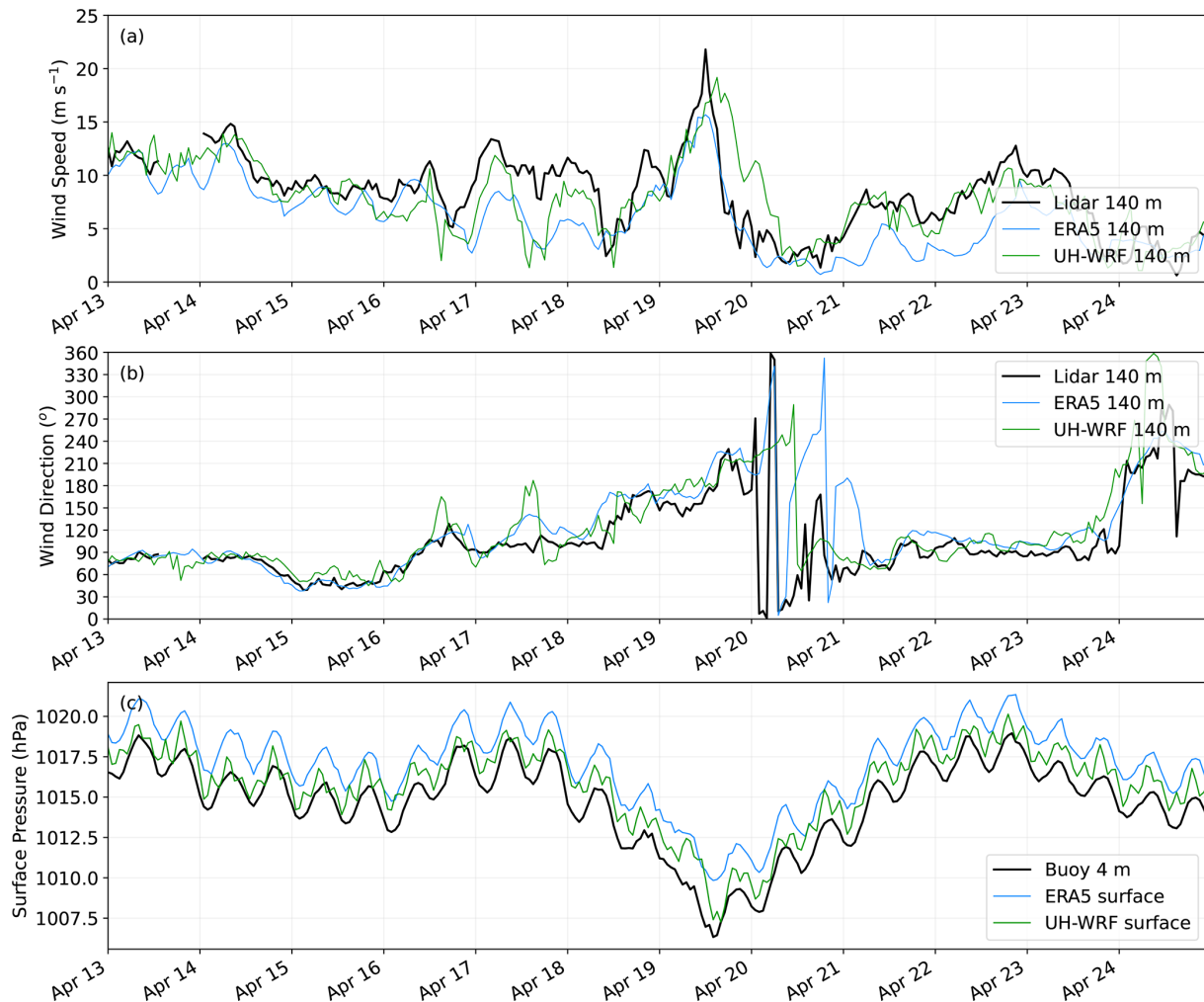
Figure 16. Observed and modelled (a) wind speeds and (b) wind directions at 140 m; (c) surface air pressures at the lidar buoy location during 13–23 April 2023 for the buoy observation, ERA5, and UH-WRF.
