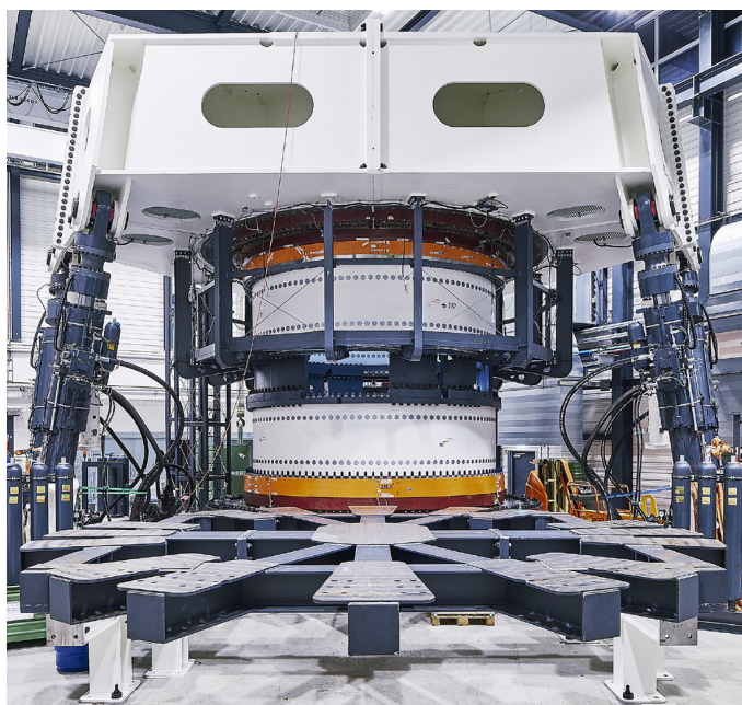
Figure 4. Fraunhofer IWES blade bearing test rig BEAT6.1 (left) and bottom view and cross-section of the lower hub adapter (right).
