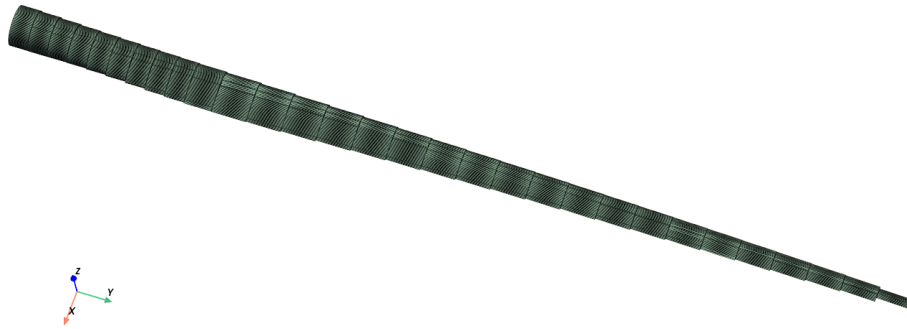
Figure 14. Structural discretization of the CRC-15-240 blade in PreDoCS.
