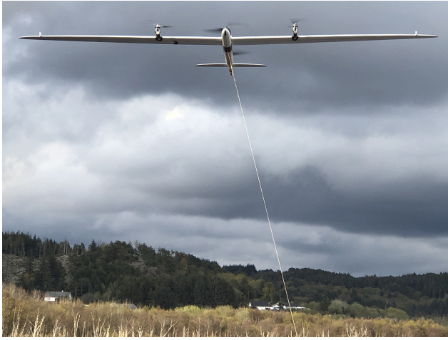
Figure 1. Aerial component of Kitemill's KM1 system.
