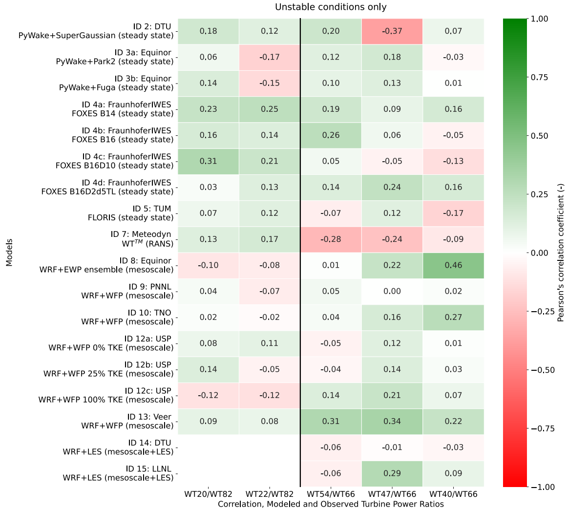
Figure S5. Pearson correlation coefficients between observed and modeled power ratios between turbine pairs during Phase 1, calculated using only data from unstable atmospheric conditions, for turbines in the western (left) and eastern (right) portions of King Plains.
