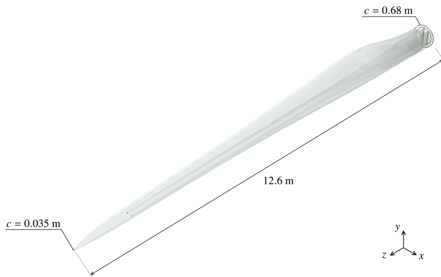
Figure 10. DTU 12.6 m wind turbine blade model. c : chord length.
