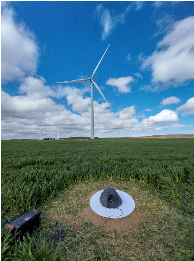
Figure 3. Picture of one SLM with E12 wind turbine in the background. The wheat crops around the SLM were cut to prevent noise disturbance. Following the recommendations of the IEC standard (IEC, 2012), all SLMs are installed on a woodboard of 1 m diameter and covered by two windscreens.
