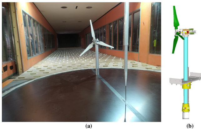
Figure 8. TWIST wind turbine model installed in the L1-B test section (a), and its CAD (b).
