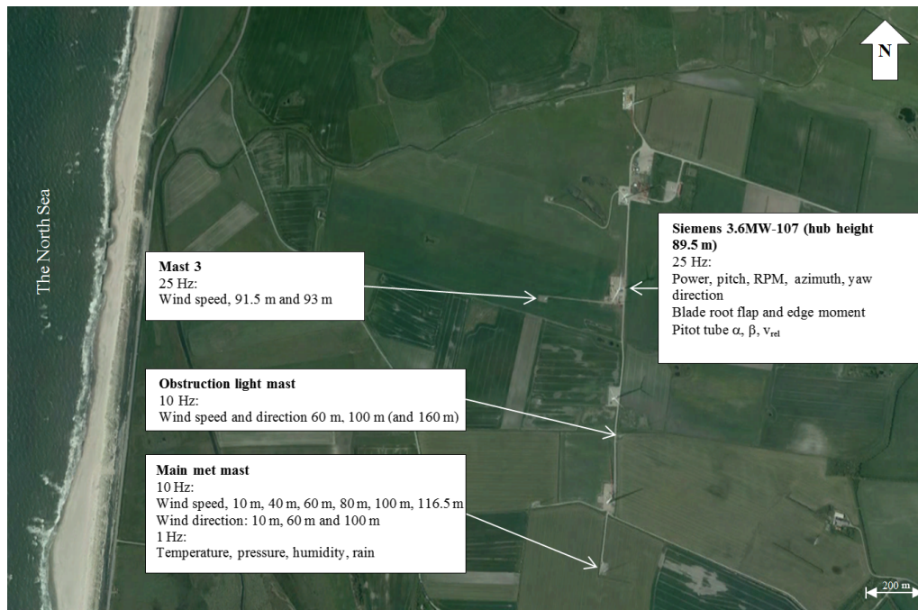
Figure 18. Overview of the Høvsøre test site for large turbines in Denmark. The Siemens turbine is located in the middle of a row of five turbines.
