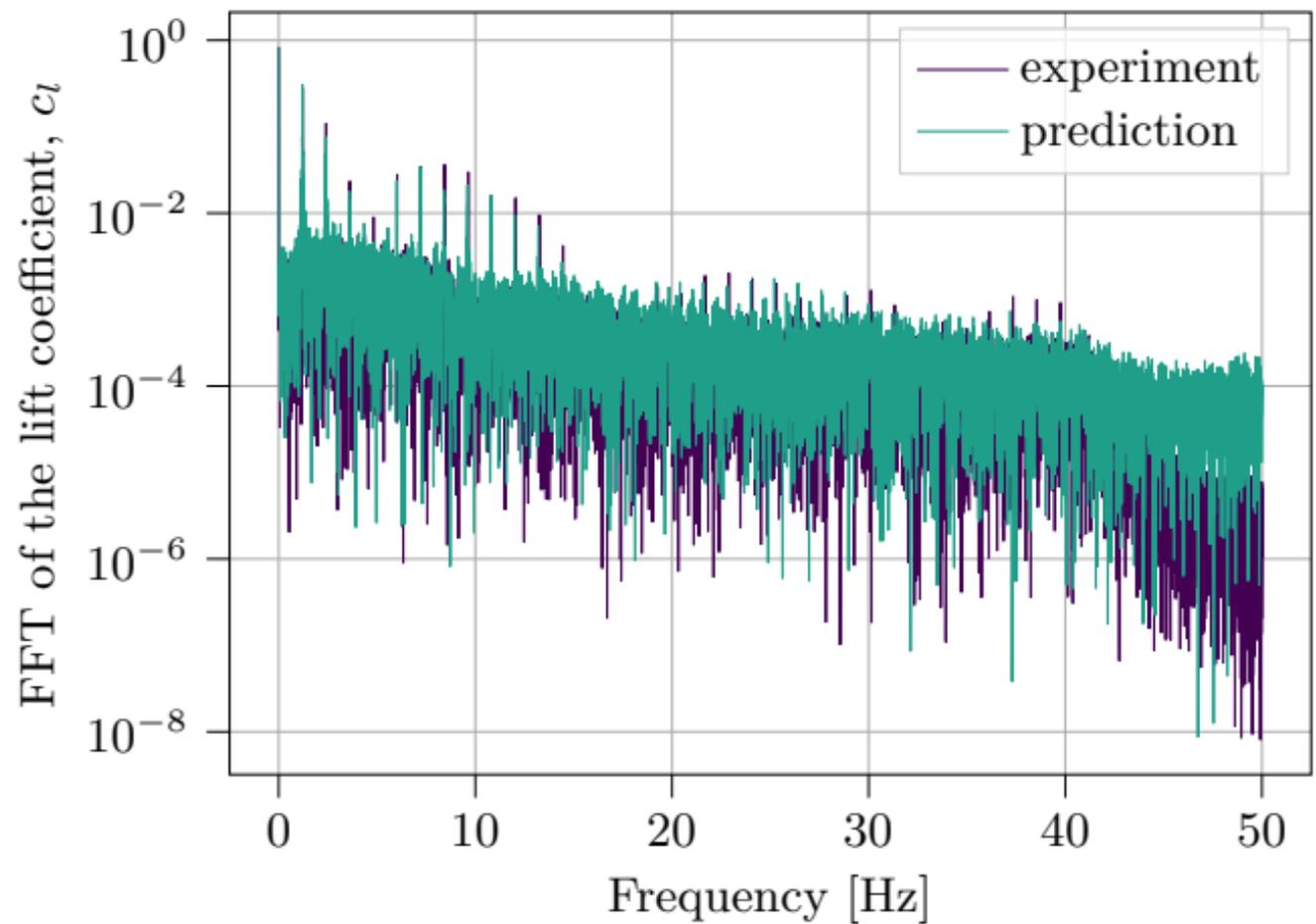
(b) Fourier transform of the lift signal
