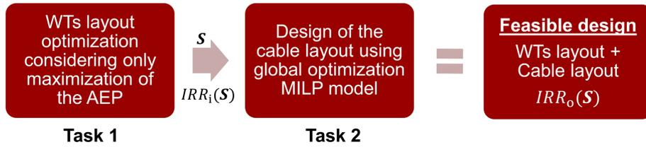
Figure 4. Approach 1: sequential design process for WTs and cable layout.
