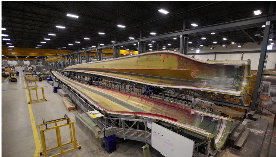
Figure 14. A 40 m wind turbine blade in production demonstrating the size and complexity of manufacturing wind turbine blades at modern scales. The assembled blade skins and internal webs are about to be bonded together, a process which has tolerances of 1 mm in some cases, and requires both speed and attention to detail for the adhesive material to bond effectively. (Photo credit: TPI Composites.)
