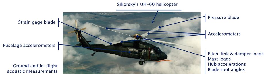
Figure 7. A highly instrumented UH-60A flying over the San Joaquin Valley in California during the UH-60A Airloads Flight Test Program. The data set collected in these experiments led to major advances in the modeling and simulation of rotorcraft vehicles. Wind energy science needs similar high-quality, fully open-access data sets, which are indispensable for validating the models and tools that will enable the design of the wind turbines of the future. (Photo from https://rotorcraft.arc.nasa.gov/Research/Programs/uh_60_program.html , last access: 19 June 2023.)
