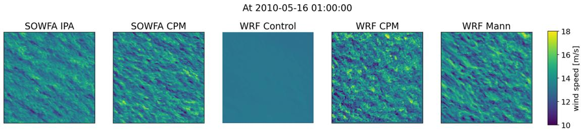
**Figure 4.** Wind speed at 01:00 local time on 16 May 2010 around the FINO1 location for the different methods investigated. The original domains contain the fetch region. Shown here is a developed-turbulence  $3 \times 3$  km subdomain.
