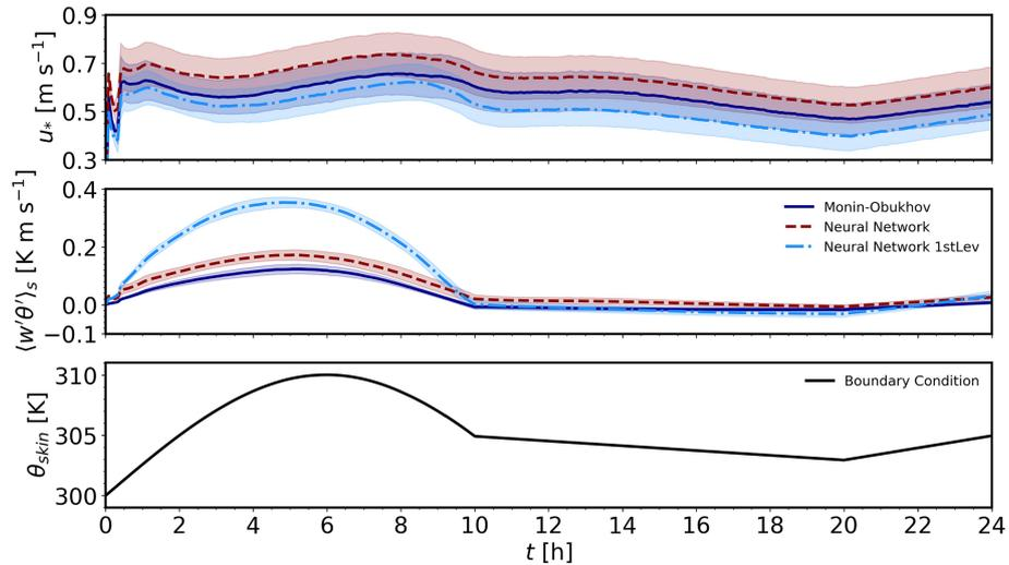
**Figure 11.** Comparison of the diurnal evolution of an ABL using the FastEddy LES model with the MOST and NN model surface-layer parameterizations: surface friction velocity (top panel), sensible heat flux (second panel), moisture flux (third panel), and boundary forcing from surface skin temperature (bottom panel). The shaded areas show 1 standard deviation from the mean over the simulation domain. Figure originally appeared in Muñoz-Esparza et al. (2022).
