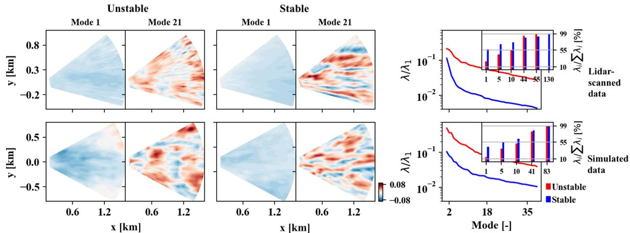
**Figure 3.** Spatial POD modes 1 and 21 for the unstable (first and second columns) and stable (third and fourth columns) condition cases and POD energy ( $\lambda$ ) among the first several modes (fifth column) and their cumulative energy (in the inset). Panels in the top and bottom rows represent the results from observed and the simulated data, respectively.
