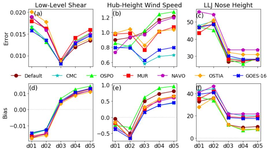
**Figure 9.** (a, b, c) Error and (d, e, f) bias for each case on each domain for (a, d) low-level shear, (b, e) hub-height wind speed, and (c, f) LLJ height. Units for error are (a, d) per second, (b, e) meters per second, and (c, f) meters.
