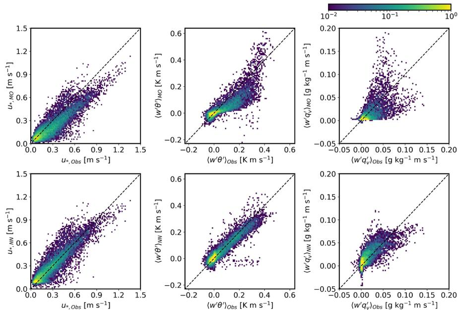
**Figure 10.** Comparison of the MOST (top row) and an offline NN model (bottom row) surface-layer parameterizations of surface friction velocity (left panels), sensible heat flux (middle panels), and moisture flux (right panels) with observations from the Cabauw mast. Figure originally appeared in Muñoz-Esparza et al. (2022).
