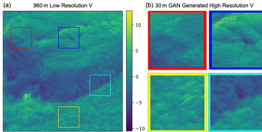
**Figure 13.** Example of using the GAN to downscale from (a) a coarsened 960 m resolution simulation to (b) four example panels showing high-resolution 30 m generated images. The colors overlaid on (a) correspond to the same color outlined image on (b).
