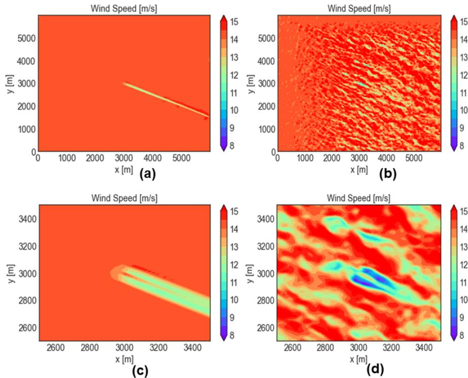
**Figure 7.** Wind speed at 01:10:00 local time on 16 May 2010 in the domain containing the turbine (AV10) location using the WRF-LES-GAD approach for (a, c) no CPM and (b, d) CPM. The entire domain is shown in (a) and (b). A subset of the domain appears in (c) and (d).
