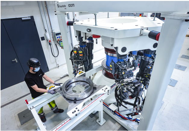
Figure 13. BEAT1.1 test rig and downscaled blade bearing 13229 (© Fraunhofer IWES/Ulrich Perrey).
