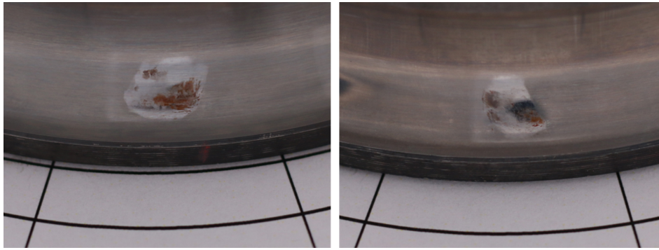
Figure 17. Wear marks on the type 7220 bearings.
