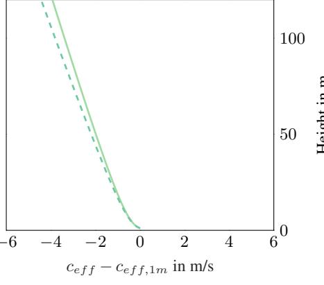
Case 9: ▲ Measurements — Modelling —  $c_{eff}$ -Profile
