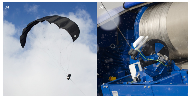
Figure 1. AWE system with (a) the 25\text{ m}^2 V3.25B kite and (b) the 100 kW ground station in operation in 2018 (photos courtesy of Kitepower B.V.).
