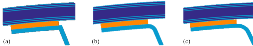
Figure 10. Cross-section detail showing range of corner radii from zero (a) through baseline (b) to 50 % larger (c).
