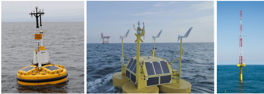
Figure 1. Photographs of the floating lidar systems (left panel: Fugro, middle panel: EOLOS) as well as the IJmuiden mast (right panel). Sources: Fugro, EOLOS and Wind op Zee.
