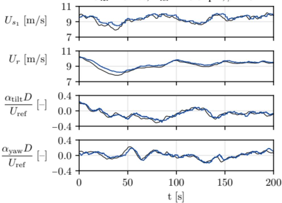
$$U_{\text{ref}} = 14 \text{ m/s}, \Omega_{\text{rot}} = 12.1 \text{ rpm}, \beta = 8.7^\circ$$
