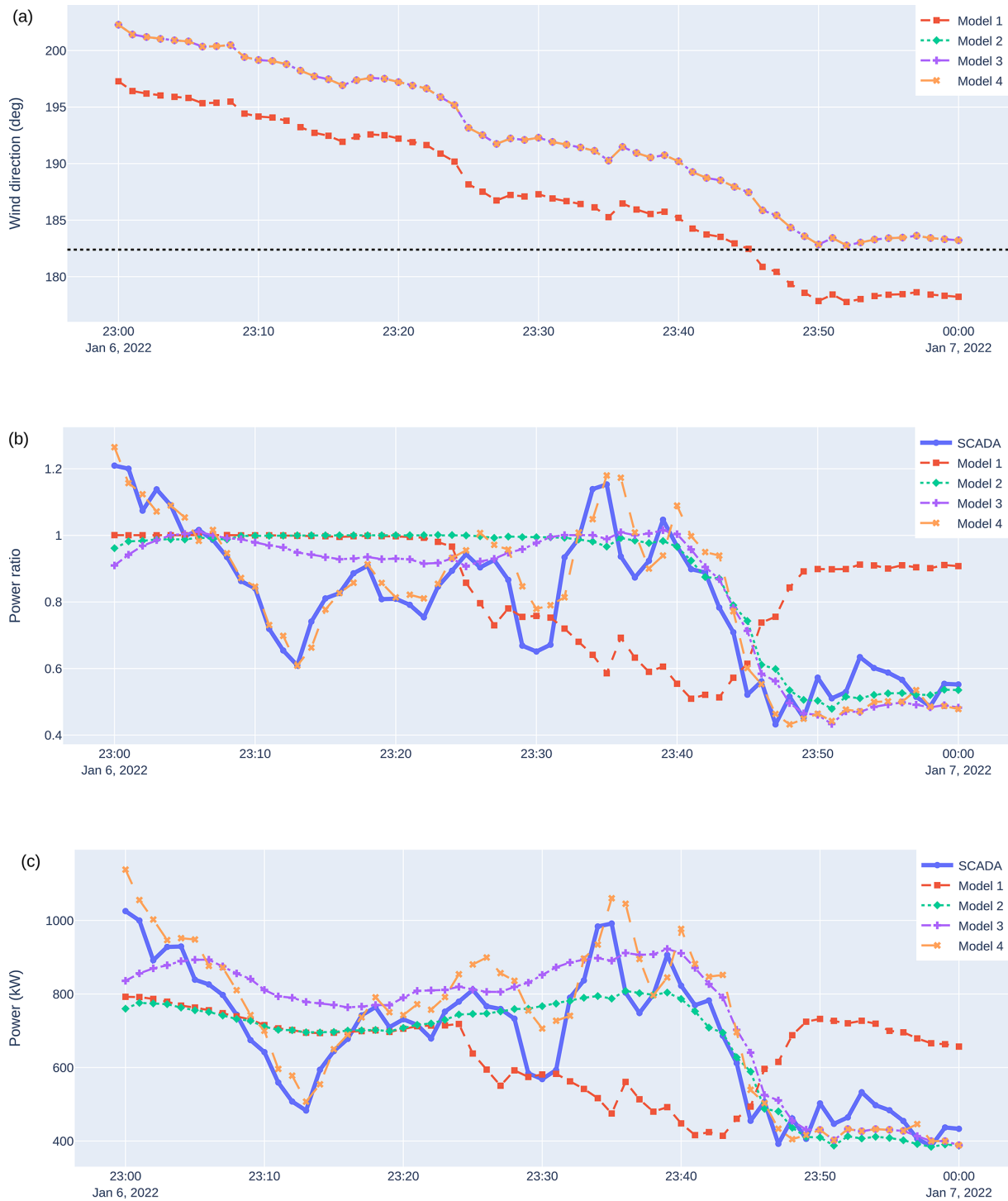
Figure 16. Example time series showing wind direction (a), power ratio (b), and power (c) for turbine 22 for a time when wake steering is disabled. SCADA results are compared against the predictions from various models from Table 1. The dotted horizontal line in (a) shows a wind direction where the downstream turbine (22) is expected to be waked by the upstream turbine (10). Several drops in power ratio occur throughout the time series, likely due to a combination of heterogeneity and waking on short timescales.
