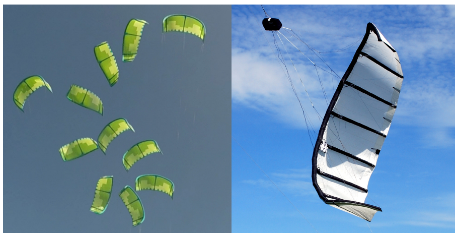
Figure 1. Time-lapse composite photo of a 6 m 2 power kite for sport applications performing a sharp turn to the left and subsequent loop manoeuvre, taken from the towing vehicle, from Lange (2018) (left panel). Photo of a 25 m 2 power kite for airborne wind energy applications performing a turn to the right during a mast-based launch manoeuvre, reported by Oehler and Schmehl (2019) (right panel). Both photos illustrate the spanwise twist deformation exhibited by LEI kites. The extreme deformation in the right photo does not occur in regular flight operations but resulted from mast-based launch attempts, shown here only to visualize the wing twist mechanism.
