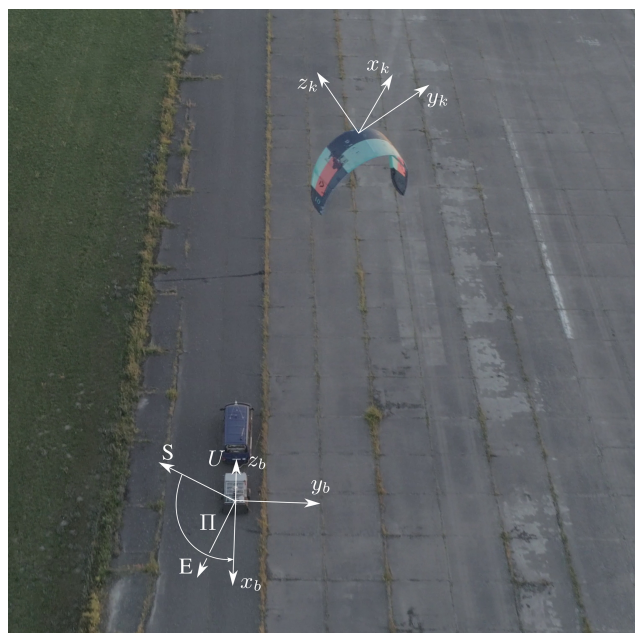
Figure 9. Kite-fixed coordinate system and test-bench-fixed coordinate system (Elfert, 2021).
