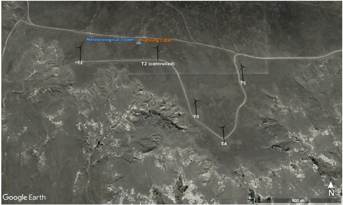
Figure 1. Site of the wake-steering field campaign, focusing on flow from the north through five turbines (T1–T5), with wake steering applied to T2 to benefit T3; inflow measurements come from a co-located meteorological tower and profiling lidar upstream. Map data from Google, © 2023 CNES/Airbus, Maxar Technologies, USDA/FPAC/GEO.
