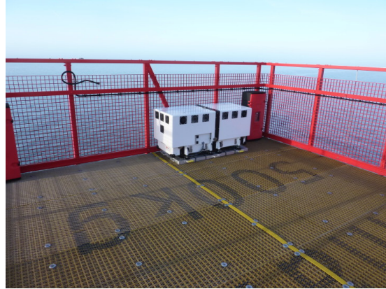
Figure 4. Measurement system installation at alpha ventus. Layout of alpha ventus wind farm and position of FINO1 meteorological mast (left). Photography of installation of Windcube plus scanner at helicopter deck of the Adwen's AD 5-116 (right).
