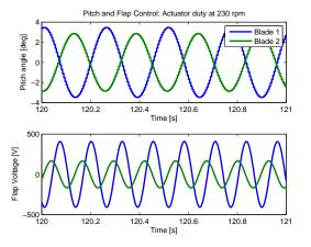
**Figure 21.** Actuator duty cycles of optimised controller (PRE-FLUTTER)
