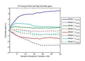
Figure 19. Convergence of controller gains over iterations
