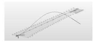
**Figure 11.** Second flapwise mode: Mode 4, Frequency 87.88 Hz
