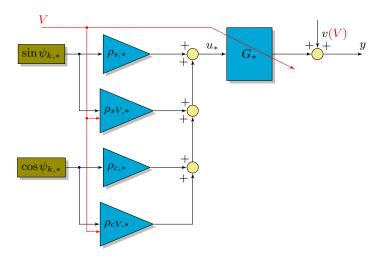
Figure 16. IFT implementation: wind turbine load control. \* stands for IPC or IFC.
