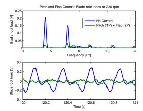
**Figure 22.** Load reductions achieved by optimised controller (PRE-FLUTTER)
