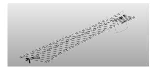
**Figure 12.** First torsional mode: Mode 7, Frequency 361.6 Hz
