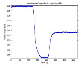
**Figure 25.** Varying operational speed for optimisation of gain schedule.
