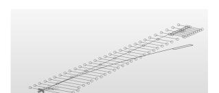
Figure 9. First flapwise mode: Mode 2, Frequency 19.44 Hz
