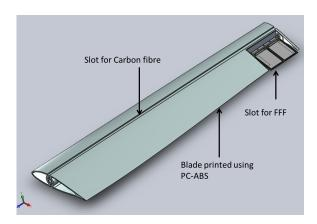
Figure 3. Blade CAD model
