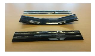
**Figure 2.** 3d printed samples post fracture. Top: ABS M30, Middle: PC-ABS, Bottom: Nylon
