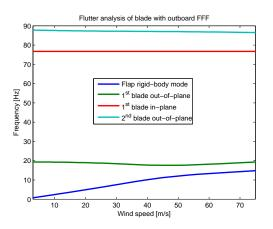
**Figure 13.** Variation in modal frequency with total incident air speed.
