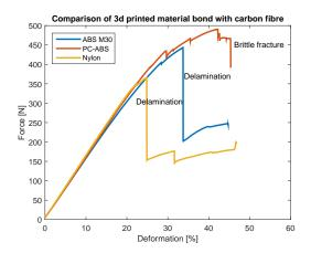
**Figure 1.** Structural behaviour of the bond between 3d printed substrate and carbon fibre spar
