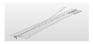
**Figure 10.** First lead-lag mode: Mode 3, Frequency 76.67 Hz
