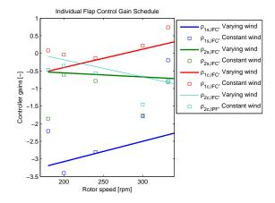
**Figure 28.** Gain schedule at varying wind speeds versus optimal gains at constant wind speed: Pitch Control.
