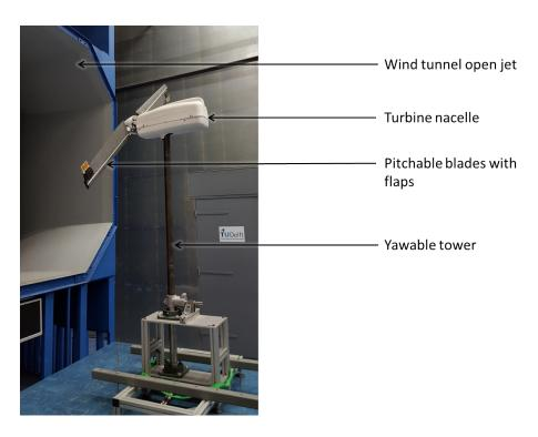
**Figure 15.** Photograph of the assembled turbine with pitch and flap control.
