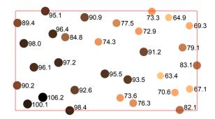
Figure 9. Optimal layout and relative power for the uniform wind-direction case (angle of  $\pm 180^{\circ}$ ). Relative power results are obtained from large-eddy simulations. Turbine locations are marked with colored disk: size and color are scaled with relative power. Plot boundary (red line) corresponds to boundaries of domain  $\Omega$  (cf. Figure 1).
