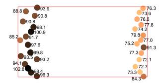
Figure 8. Optimal layout and relative power for dominant wind-direction case (angle of  $\pm 7.5^{\circ}$ ). Relative power results are obtained from large-eddy simulations. Turbine locations are marked with colored disk: size and color are scaled with relative power. Plot boundary (red line) corresponds to boundaries of domain  $\Omega$  (cf. Figure 1).
