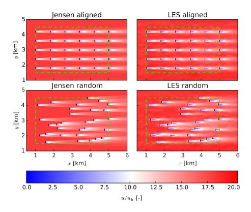
Figure 4. Comparison of Jensen Model and LES for an aligned and random layout.
