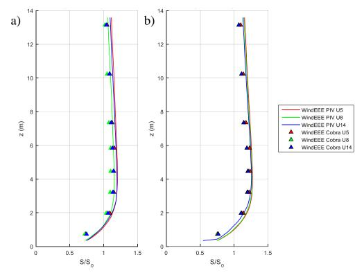
Figure 9. WindEEE PIV and Cobra Probe vertical profiles of speed-up ratio at M6, for RC1 (left) and RC2 (right).
