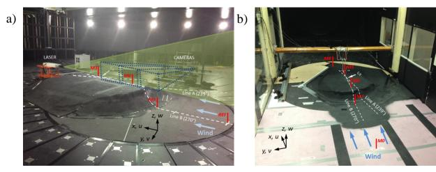
Figure 1. Experimental setup for a) WindEEE b) BLWTL.
