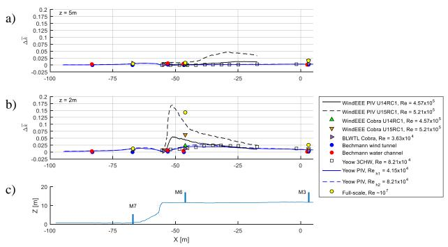
**Figure 11.** WindEEE and BLWTL TKE increment along horizontal profiles at a) z = 5m and b) z = 2m above surface level for PIV and Cobra Probe measurements with comparison to full-scale and to previous physical experiments.
