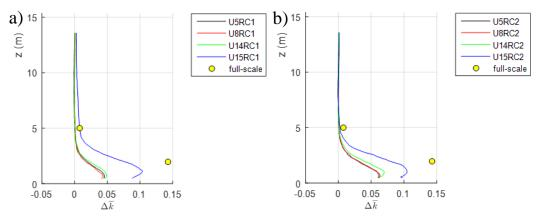
Figure 14. Vertical profiles of TKE increment at M6 for a) RC1 cases and b) RC2 cases.
