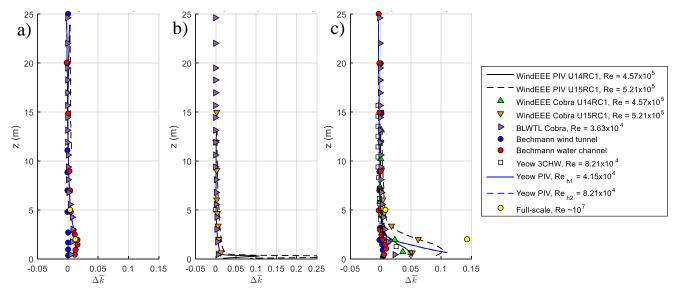
Figure 12. Comparison of WindEEE and BLWTL TKE increment along vertical profiles at a) M7 (X = -66.9 m), b) escarpment (X = -54.7 m) and c) M6 (X = -46.1 m) with comparison to full-scale and to previous physical experiments.
