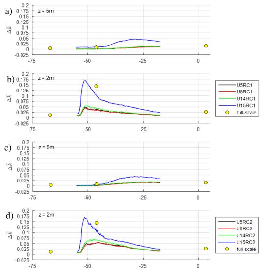
**Figure 13.** Change in TKE horizontal profiles for a) RC1 cases at z = 5 m. and b) RC1 cases at z = 2 m, c) RC2 cases at z = 5 m, and d) RC2 cases at z = 2 m.
