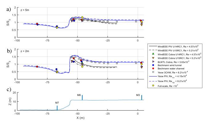
**Figure 5.** WindEEE and BLWTL speed-up ratio along horizontal profiles at a) z = 5 m and b) z = 2 m above surface level for PIV and Cobra Probe measurements with comparison to full-scale and to previous physical experiments.
