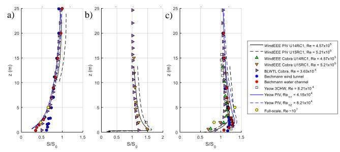
**Figure 6.** Comparison of WindEEE and BLWTL speed-up ratio along vertical profiles at a) M7 (X = -66.9 m), b) escarpment (X = -54.7 m) and c) M6 (X = -46.1 m) with comparison to full-scale and to previous physical experiments.
