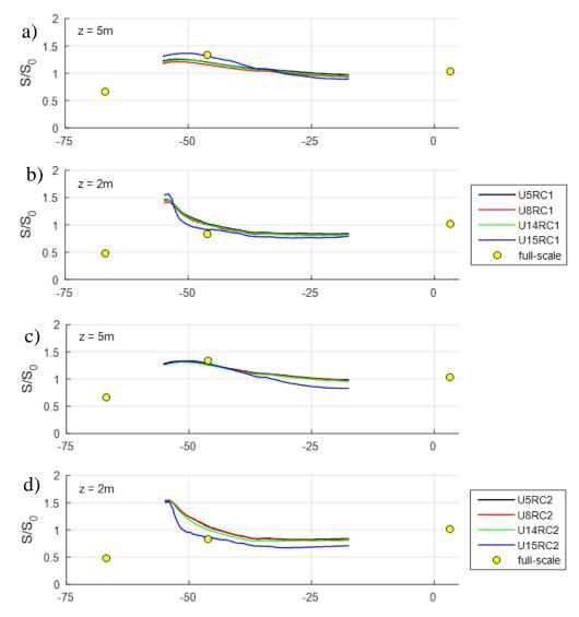
**Figure 7.** Horizontal profiles of speed-up ratio for a) RC1 cases, z = 5 m, b) RC1 cases, z = 2 m, c) RC2 cases, z = 5 m and d) RC2 cases, z = 5 m.
