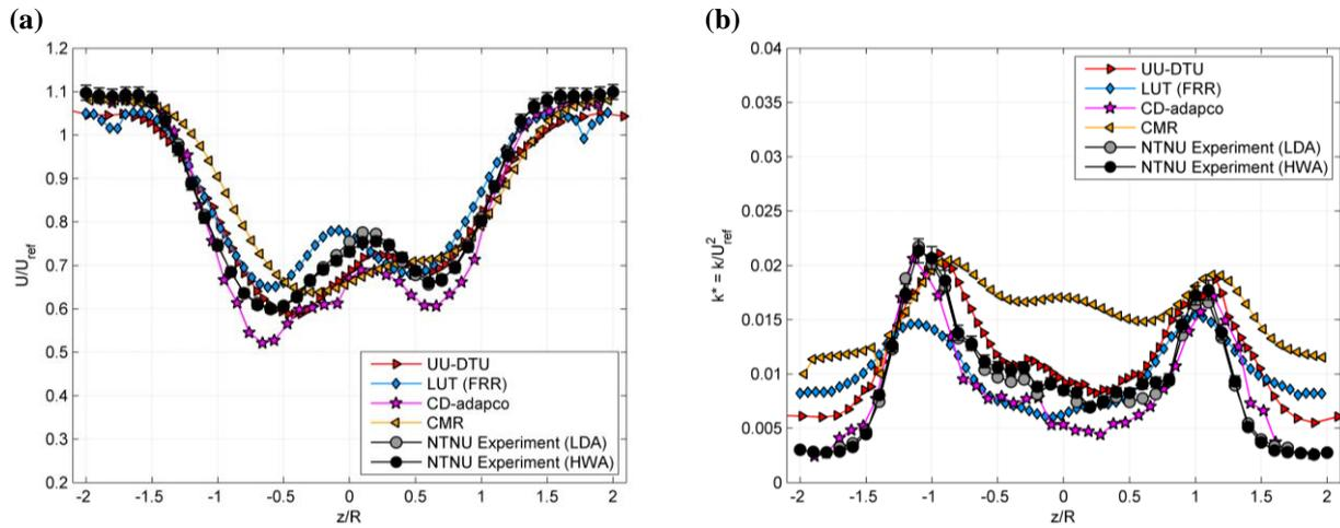
**Figure 10.** Normalized mean velocity  $U/U_{ref}$  (a) and normalized turbulent kinetic energy  $k/U_{ref}^2$  (b) in the wake  $x/D=2.77$  behind T1 measured for test case C. The upstream turbine T1 is operated at  $\lambda_{T1}=6.0$ . The reference velocity  $U_{ref} = 11.5\text{m/s}$  is the velocity experienced by T1 at hub height.
