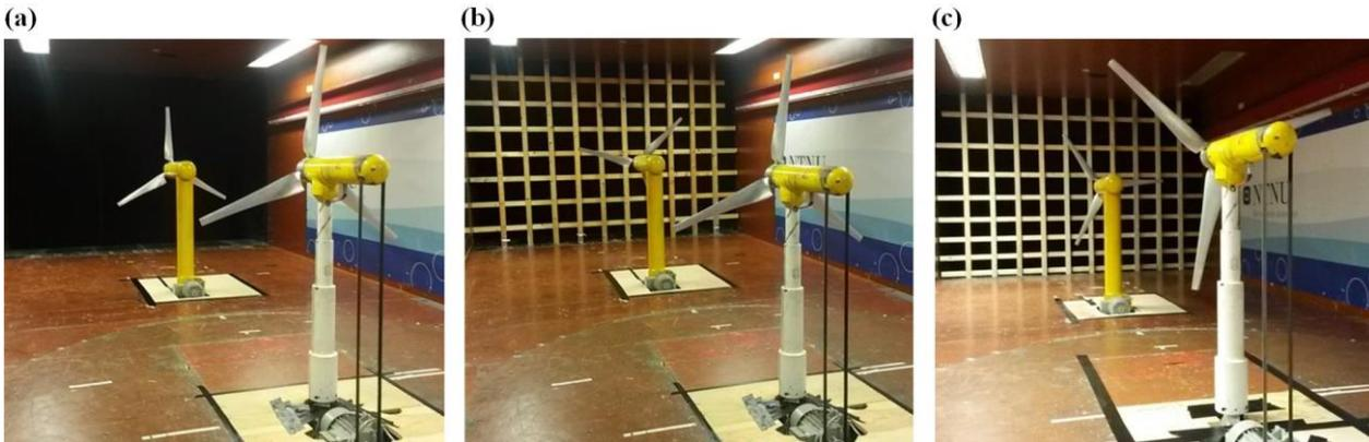
**Figure 4.** Test case A: low turbulence uniform inflow (a); test case B: high turbulence uniform inflow (b); test case C: high turbulence shear inflow (c).
