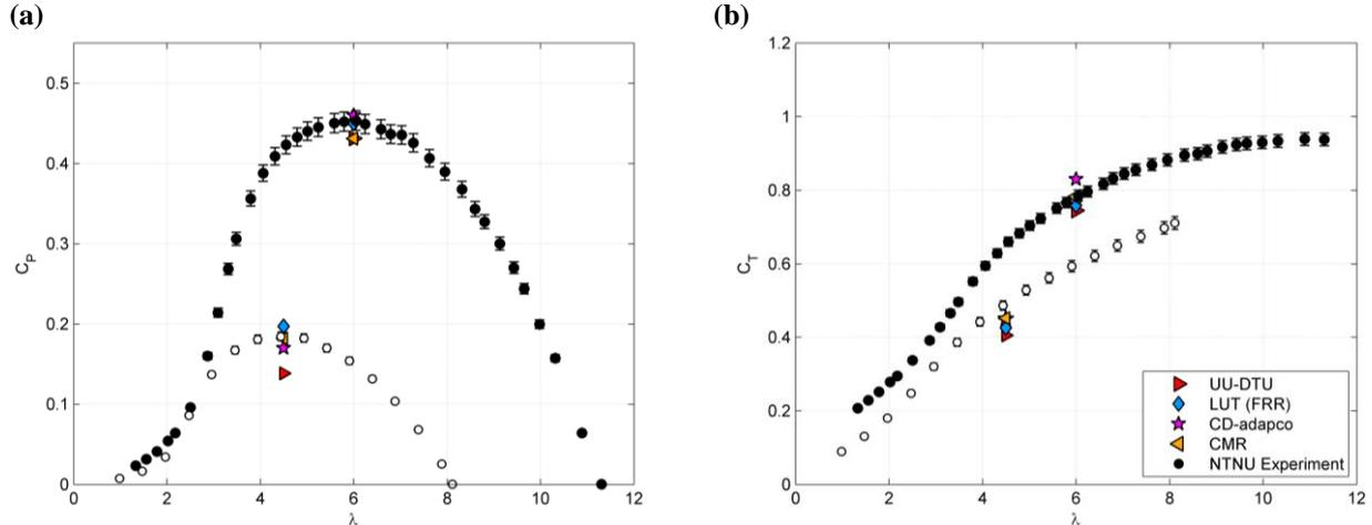
**Figure 9.** Power coefficient  $C_p$  (a) and Thrust coefficient  $C_T$  (b) for T1 (filled symbols) and T2 (empty circles) compared for test case C. The downstream turbine T2 is positioned at  $x/D=5.18$  downstream of T1 and the upstream turbine T1 is operated at  $\lambda_{T1}=6.0$ . The reference velocity  $U_{ref} = 11.5\text{m/s}$  is the velocity experienced by T1 at hub height.
