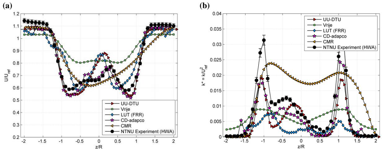
**Figure 6.** Normalized mean velocity  $U/U_{ref}$  (a) and normalized turbulent kinetic energy  $k^*/U_{ref}$  (b) in the wake  $x/D=2.77$  behind T1 measured for test case A. The upstream turbine T1 is operated at  $\lambda_{T1}=6.0$ . The reference velocity is  $U_{ref} = 11.5$  m/s.
