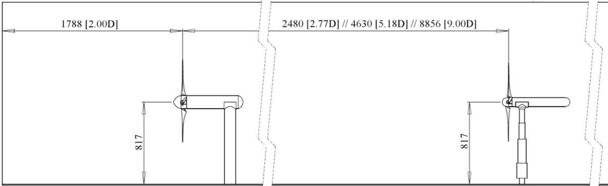
**Figure 3.** Setup of the model wind turbine in the wind tunnel.
