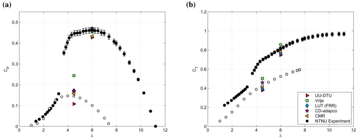
**Figure 5.** Power coefficient  $C_p$  (a) and Thrust coefficient  $C_T$  (b) for T1 (filled circles) and T2 (empty circles) compared for test case A. The downstream turbine T2 is positioned at  $x/D=5.18$  downstream of T1 and the upstream turbine T1 is operated at  $\lambda_{T1}=6.0$ . The reference velocity is  $U_{ref} = 11.5$  m/s.
