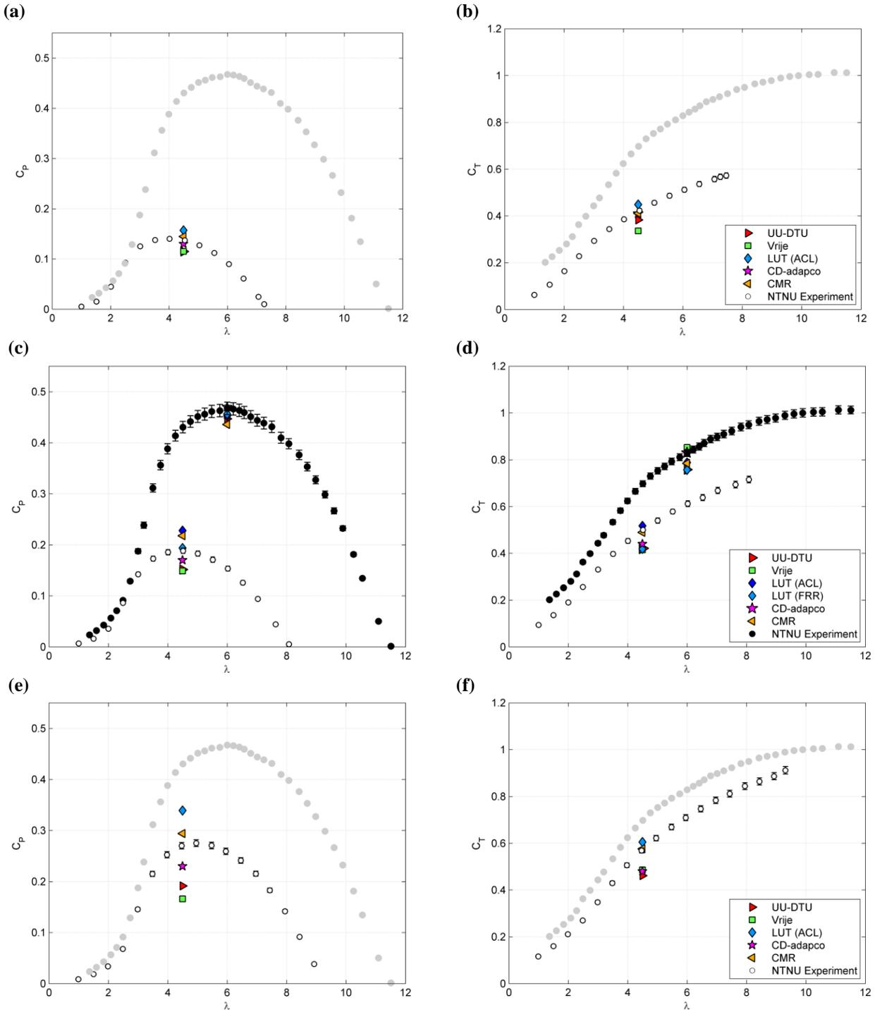
**Figure 7.** Power coefficient  $C_p$  (a, c, e) and Thrust coefficient  $C_T$  (b, d, f) for T1 (filled symbols) and T2 (empty circles) compared for test case B<sub>1</sub>, B<sub>2</sub> and B<sub>3</sub>. The downstream turbine T2 is positioned at  $x/D=2.77$  (a, b), 5.18 (c, d) and 9.00 (e, f) downstream of T1. The upstream turbine T1 is operated at  $\lambda_{T1}=6.0$ . The reference velocity is  $U_{ref} = 11.5\text{m/s}$ .
