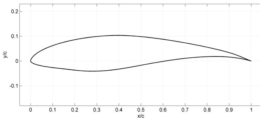
**Figure 2.** NREL S826 airfoil geometry.
