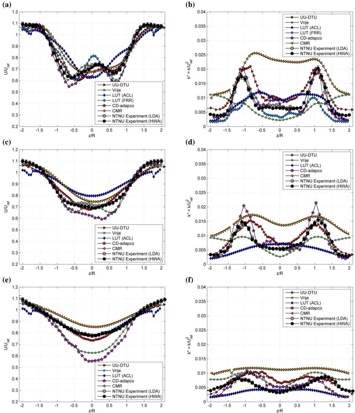
**Figure 8.** Normalized mean velocity  $U/U_{ref}$  (a, c, e) and normalized turbulent kinetic energy  $k/U_{ref}^2$  (b, d, f) in the wake  $x/D=2.77$  (a, b), 5.18 (c, d) and 8.50 (e, f) behind T1 for test case setup B<sub>3</sub>. The upstream turbine T1 is operated at  $\lambda_{T1}=6.0$ . The reference velocity is  $U_{ref} = 11.5\text{m/s}$ .
