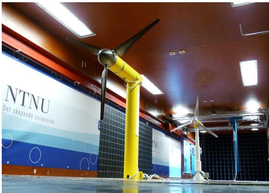
**Figure1.** Model wind turbines ( $x/D=2.77$ ) installed in the test section of NTNU's low speed wind tunnel.
