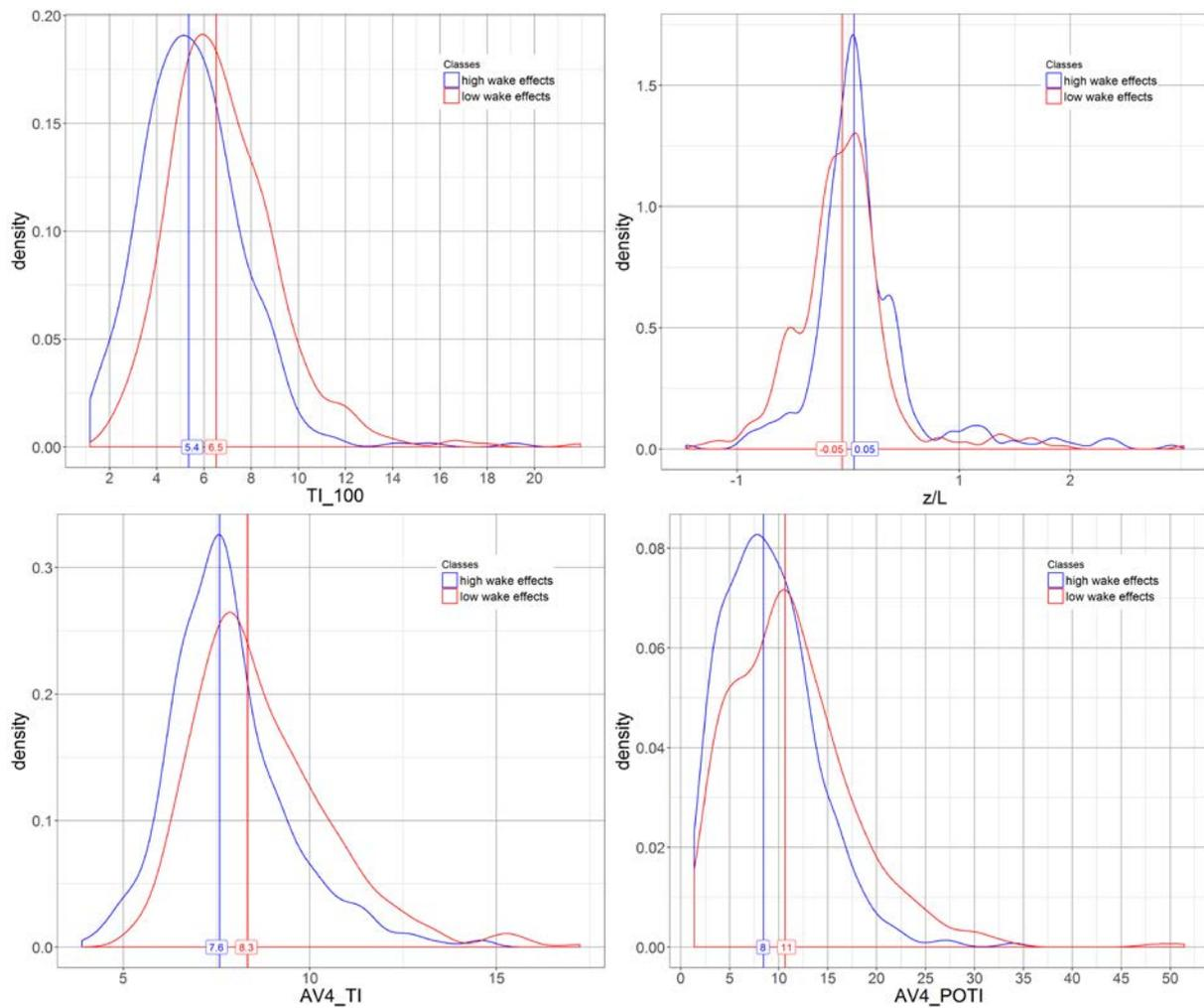
Fig 2. Data density for different variables based on low and high wake effects. The median for each distribution is highlighted with a vertical line. The data corresponds to a wind speed bin of  $8 \pm 1$  m/s and a sector width of  $10^\circ$  around the full wake.
