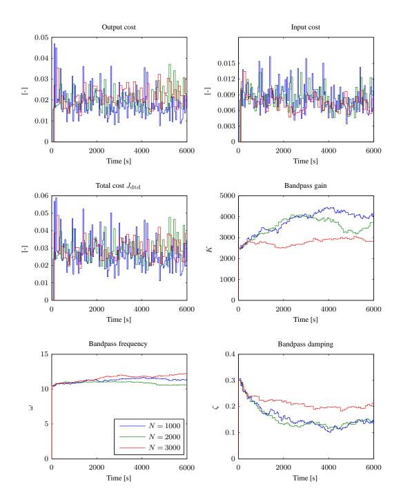
Figure 12. Comparison of IFT performance for different number N of collected data samples. Result shown are obtained with  $\gamma = 0.3$ ,  $\lambda = 5 \cdot 10^{-7}$ , F = 2000, and turbulent wind with mean speed 14 m s<sup>-1</sup> and 10% turbulence intensity.
