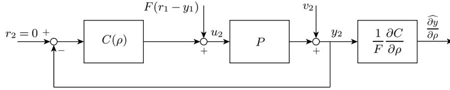
**Figure 2.** Block diagram of the closed-loop gradient experiment.
