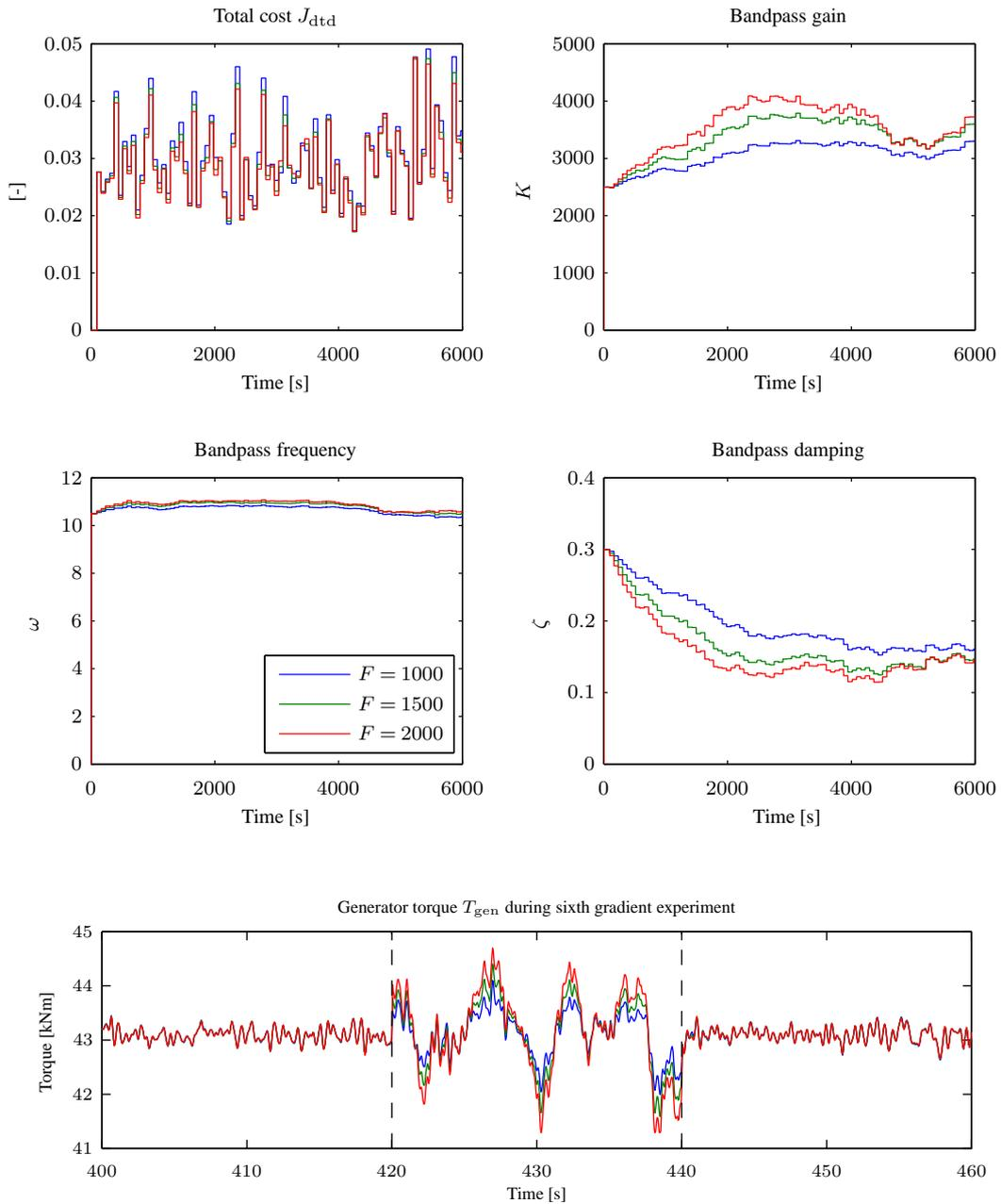
**Figure 11.** Comparison of three different signal-to-noise ratio scaling factors  $F$ . Results are shown for  $\gamma = 0.3$ ,  $\lambda = 5 \cdot 10^{-7}$ , and turbulent wind with mean speed  $14 \text{ m s}^{-1}$  and 10% turbulence intensity.
