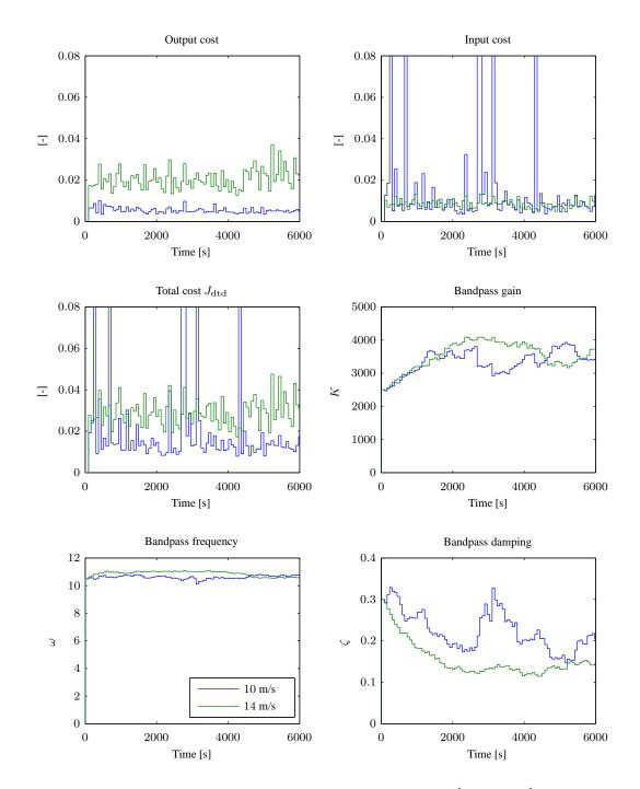
Figure 13. Comparison of IFT performance for turbulent wind with mean wind speeds  $10 \text{ m s}^{-1}$  and  $14 \text{ m s}^{-1}$ , both with 10% turbulence intensity. Results shown are obtained with  $\gamma = 0.3$  and  $\lambda = 5 \cdot 10^{-7}$ .
