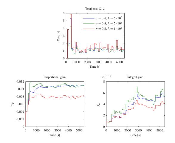
Figure 14. Reference step tuning using IFT of CPC at a wind speed of  $14 \text{ m s}^{-1}$  with 4% turbulence intensity.. The results show three different cases where the step size  $\gamma$  and the input weighting  $\lambda$  in the cost function are varied.
