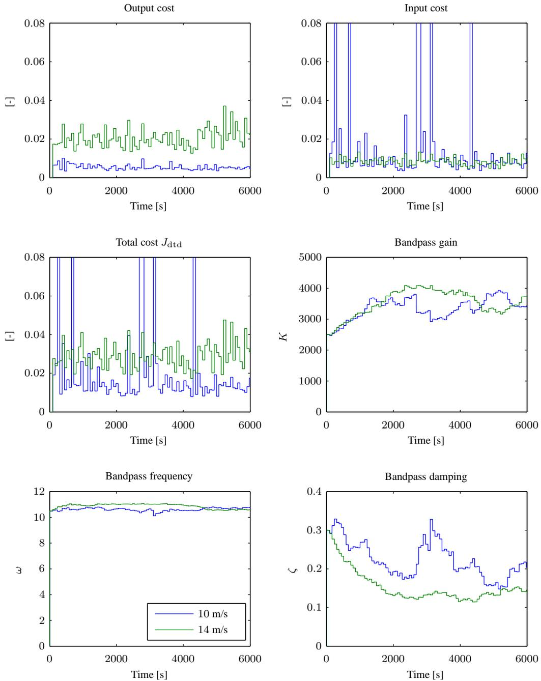
**Figure 13.** Comparison of IFT performance for turbulent wind with mean wind speeds  $10 \text{ m s}^{-1}$  and  $14 \text{ m s}^{-1}$ , both with 10% turbulence intensity. Results shown are obtained with  $\gamma = 0.3$  and  $\lambda = 5 \cdot 10^{-7}$ .
