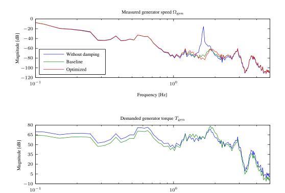
Figure 10. Comparison of the baseline and IFT optimized drivetrain controller performance.
