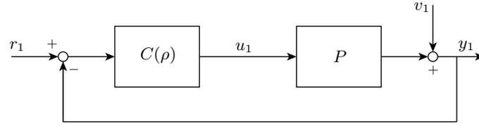
**Figure 1.** Block diagram of a closed-loop system.
