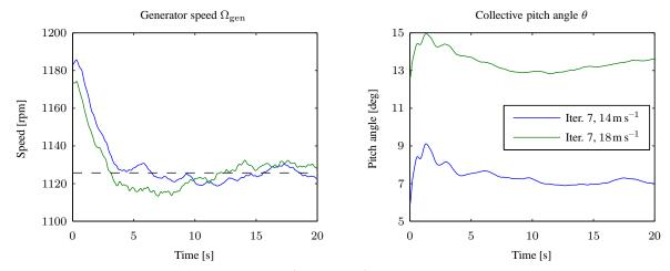
Figure 18. Comparison of the CPC step responses for  $14 \text{ m s}^{-1}$  and  $18 \text{ m s}^{-1}$  with 4% turbulence intensity during the seventh iteration.
