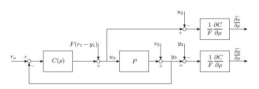
Figure 3. Block diagram of modified closed-loop gradient experiment for reference inputs with offsets.
