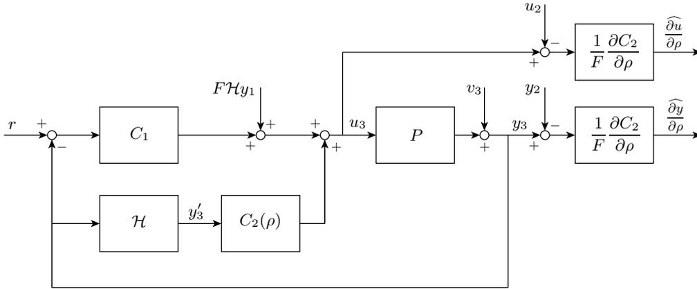
**Figure 5.** Block diagram of the gradient experiment for the multiple controller scenario. The controller  $C_1$  is fixed and controller  $C_2(\rho)$  is subject to IFT. The signals  $\mathcal{H}y_1(k, \rho)$ ,  $y_2(k, \rho)$  and  $u_2(k, \rho)$  are obtained from two others experiments and are required to obtain unbiased gradient estimates.
