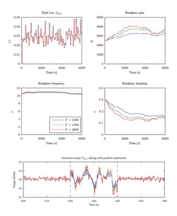
Figure 11. Comparison of three different signal-to-noise ratio scaling factors F. Results are shown for  $\gamma = 0.3$ ,  $\lambda = 5 \cdot 10^{-7}$ , and turbulent wind with mean speed 14 m s<sup>-1</sup> and 10% turbulence intensity.
