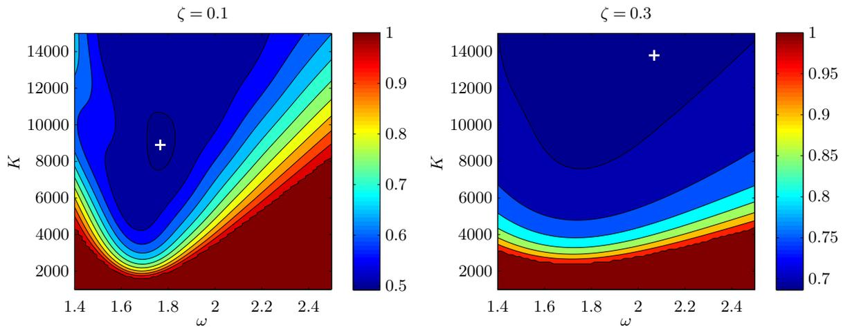
**Figure 8.** Close-up of the optimal parameter combinations for the drivetrain excitation problem with  $\zeta = 0.1$  (left) and  $\zeta = 0.3$  (right). The results are thresholded and normalized for clarity. The results show large areas where the cost function is almost optimal. The minimum values of the cost function for each case is indicated by the white + marker.
