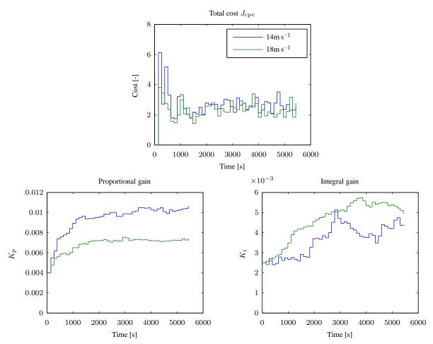
Figure 17. Reference step tuning of CPC using IFT of CPC at a wind speed of 14 m s<sup>-1</sup> with 4% turbulence intensity...
