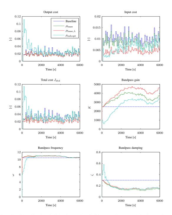
Figure 9. Comparison of three drivetrain torsional damping controllers of which two are subject to IFT. The baseline controller parameters are kept constant and the result is shown as reference. The other three cases involve IFT where the torsional damper is optimized starting from different initial conditions. Results shown are obtained with  $\gamma = 0.3$ , F = 2000, and turbulent wind with mean speed  $14 \text{ m s}^{-1}$  and 10% turbulence intensity.
