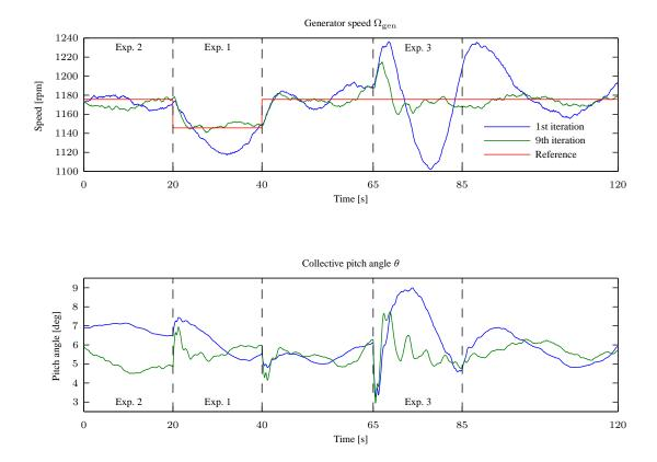
**Figure 16.** Comparison of responses during first and ninth iteration. Results shown are obtained for a wind speed of  $14 \text{ m s}^{-1}$  with 4% turbulence intensity. The measured generator speed and reference input are shown in the upper plot, the lower plot displays the pitch response.
