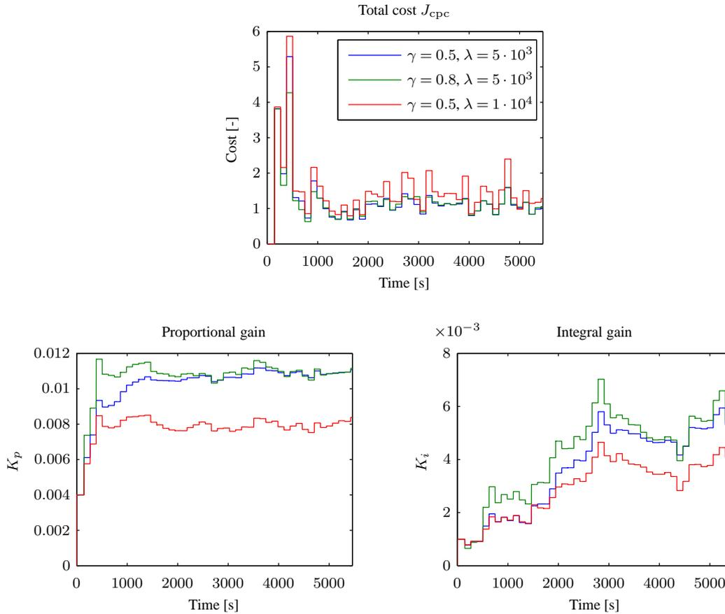
**Figure 14.** Reference step tuning using IFT of CPC at a wind speed of  $14 \text{ m s}^{-1}$  with 4% turbulence intensity.. The results show three different cases where the step size  $\gamma$  and the input weighting  $\lambda$  in the cost function are varied.
