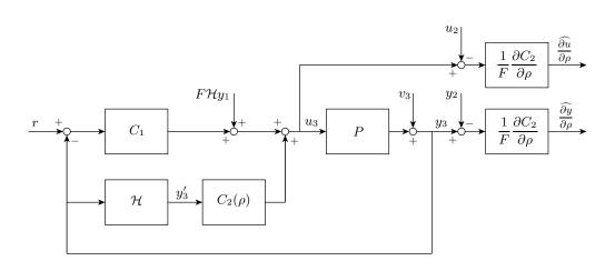
Figure 5. Block diagram of the gradient experiment for the multiple controller scenario. The controller  $C_1$  is fixed and controller  $C_2(\rho)$  is subject to IFT. The signals  $\mathcal{H}y_1(k,\rho)$ ,  $y_2(k,\rho)$  and  $u_2(k,\rho)$  are obtained from two others experiments and are required to obtain unbiased gradient estimates.
