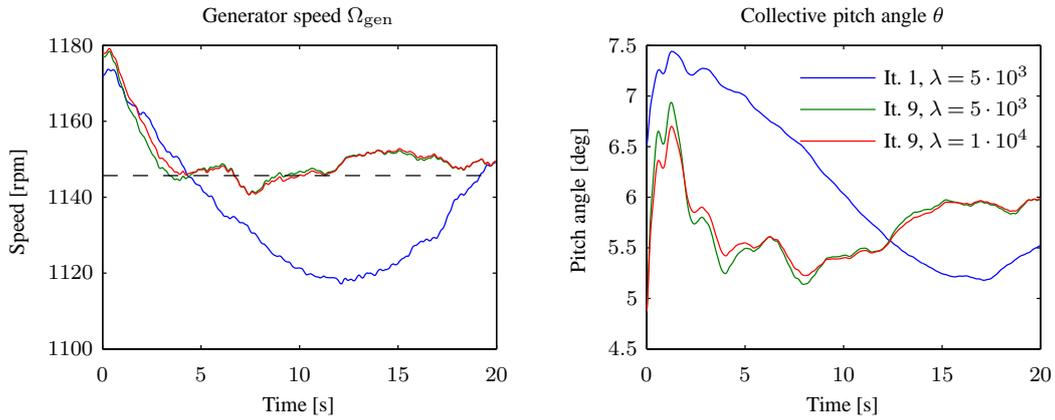
**Figure 15.** Comparison of the generator speed step response during first and ninth iteration, and for different input weighting factors  $\lambda$ . Results shown are obtained for a wind speed of  $14 \text{ m s}^{-1}$  with 4% turbulence intensity.
