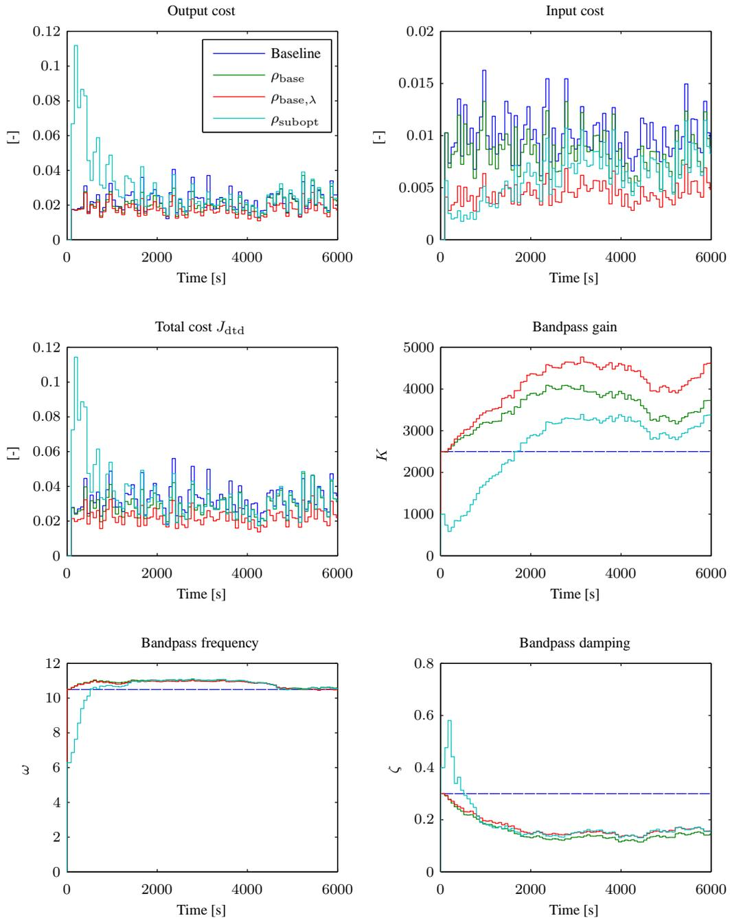
**Figure 9.** Comparison of three drivetrain torsional damping controllers of which two are subject to IFT. The baseline controller parameters are kept constant and the result is shown as reference. The other three cases involve IFT where the torsional damper is optimized starting from different initial conditions. Results shown are obtained with  $\gamma = 0.3$ ,  $F = 2000$ , and turbulent wind with mean speed  $14 \text{ m s}^{-1}$  and 10% turbulence intensity.
