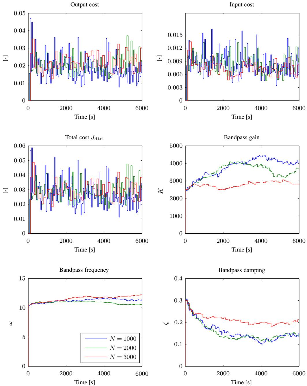
**Figure 12.** Comparison of IFT performance for different number  $N$  of collected data samples. Result shown are obtained with  $\gamma = 0.3$ ,  $\lambda = 5 \cdot 10^{-7}$ ,  $F = 2000$ , and turbulent wind with mean speed  $14 \text{ m s}^{-1}$  and 10% turbulence intensity..
