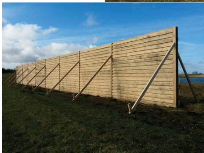
Figure 3. Photographs of the fence experiment. (Top) overview of the fence and the instrumentation including the lidars and the mast. (Left) solid and (right) porous fence setups
