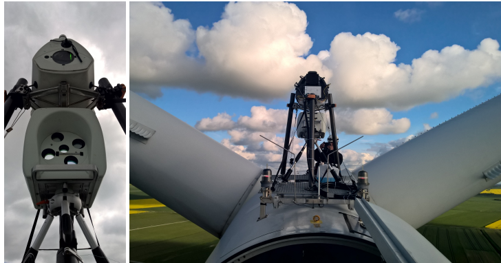
Figure 4. Measurement campaign in Nørrekær Enge (Denmark): the 5-beam Avent Demonstrator (bottom) and ZephIR Dual-Mode (top) lidars mounted on a Siemens 2.3 MW turbine.
