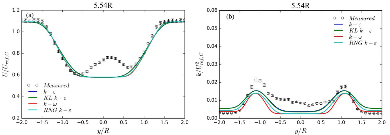
**Figure 12.** (a) Normalised axial velocity and (b) normalised turbulent kinetic energy computed for the two in-line model wind turbines (case C2) at  $x/R=5.54$  downstream of the first wind turbine. Different turbulence models are used along with the undistributed thrust.
