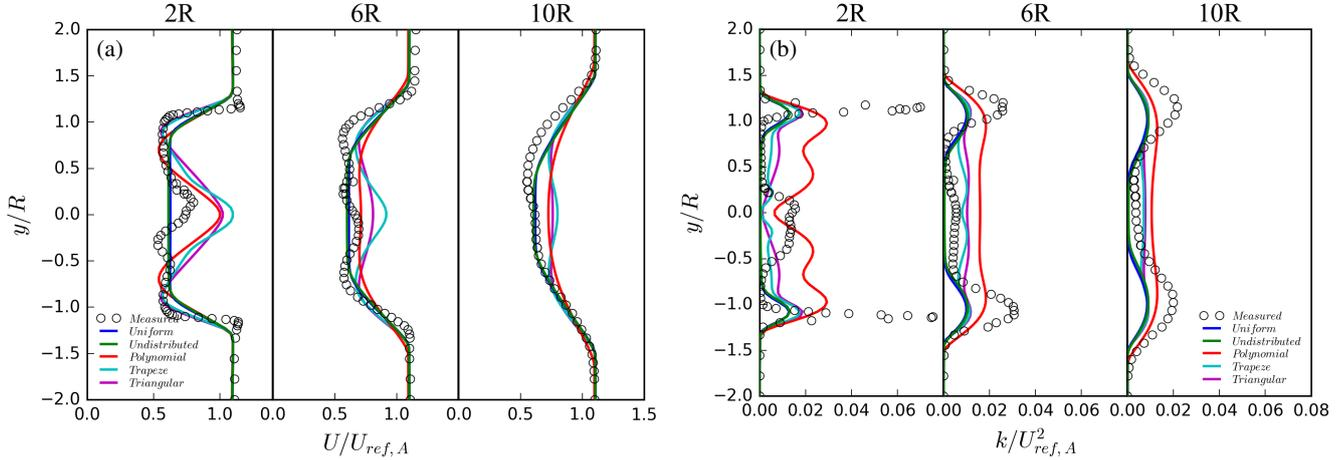
**Figure 6.** (a) Normalised axial velocity and (b) normalised turbulent kinetic energy computed behind a single model wind turbine (case A) at  $x/R = 2, 6$  and  $10$  for different thrust distributions and the  $k - \epsilon$  turbulence model.
