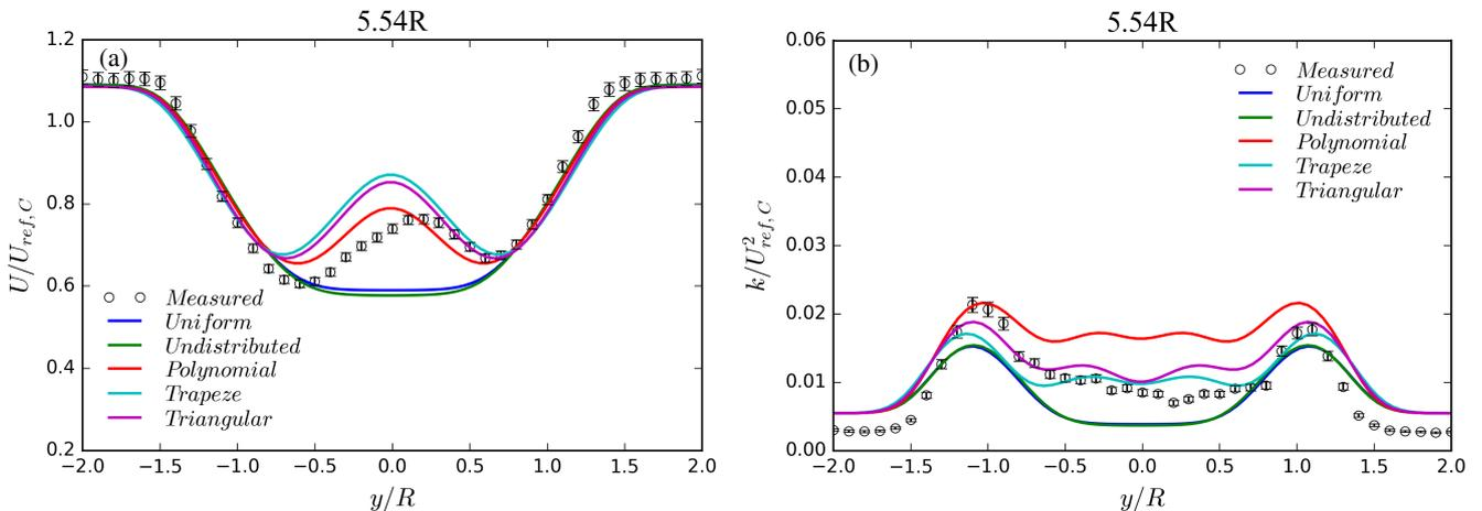
**Figure 13.** (a) Normalised axial velocity and (b) normalised turbulent kinetic energy computed for the two in-line model wind turbines (case C2) at  $x/R=5.54$  downstream of the first wind turbine. Different thrust distributions are used and the  $k-\epsilon$  turbulence model.
