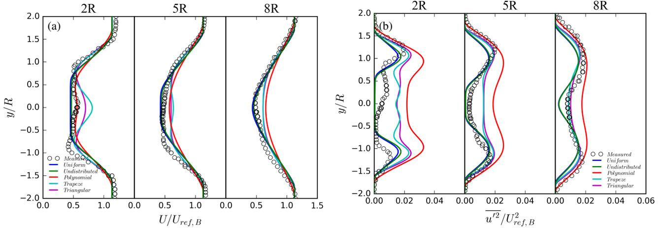
**Figure 8.** (a) Normalised axial velocity and (b) normalised stream-wise variance of the velocity computed for the two in-line model wind turbines (case B) at  $x/R = 2, 5$  and  $8$  downstream of the second wind turbine for different thrust distributions and the  $k - \varepsilon$  turbulence model.
