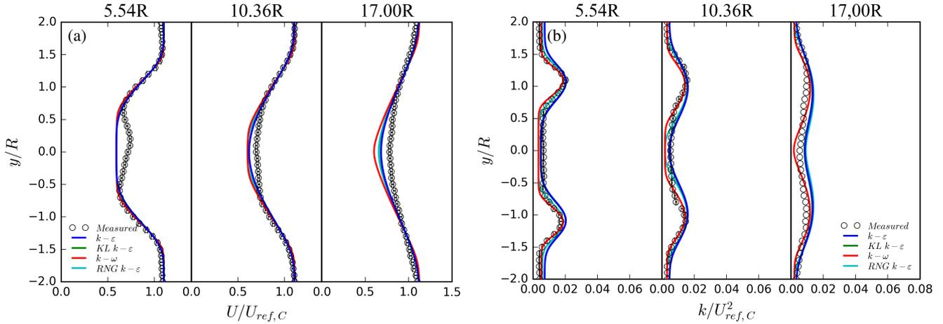
**Figure 10.** (a) Normalised axial velocity and (b) normalised turbulent kinetic energy computed for the two in-line model wind turbines (case C1) at  $x/R = 5.54, 10.36$  and  $17.00$  downstream of the first wind turbine for a separation distance of  $18.00R$ . Different turbulence models are used along with the undistributed thrust.
