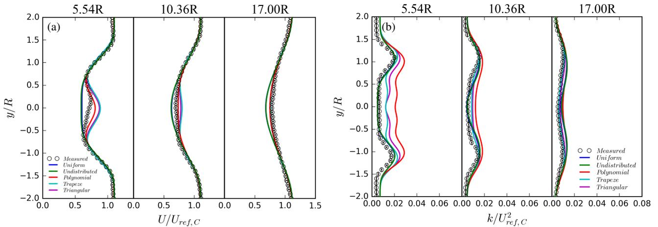
**Figure 11.** (a) Normalised axial velocity and (b) normalised turbulent kinetic energy computed for the two in-line model wind turbines (case C1) at  $x/R = 5.54, 10.36$  and  $17.00$  downstream of the first wind turbine. Different thrust distributions are used and the  $k-\epsilon$  turbulence model.
