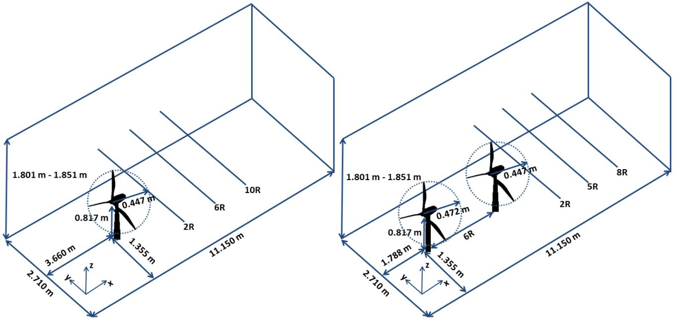
**Figure 1.** Illustration of wind tunnel layout for (a) one model wind turbine set-up (case A), (b) two in-line model wind turbine set-up (case B). The three downstream positions  $x/R = 2, 6, 10$  and  $x/R = 2, 5, 8$  are where the measurements are extracted, radius  $R = 0.447$  m.
