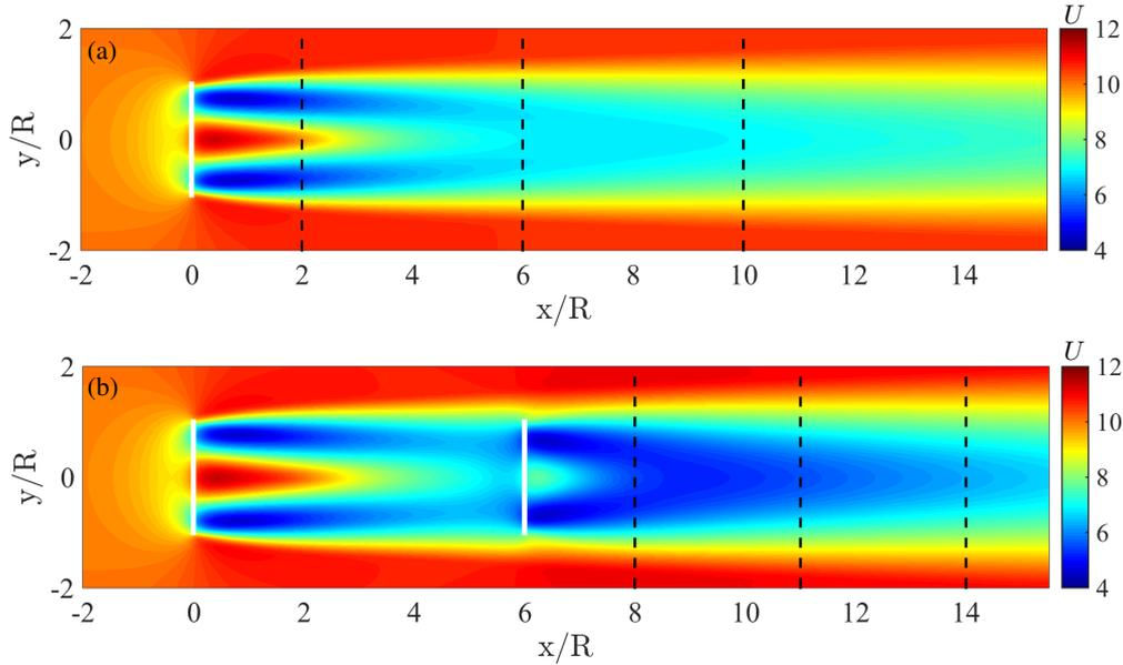
**Figure 4.** Axial velocity contours for the  $k - \epsilon$  turbulence model using the polynomial thrust distribution. (a) One model wind turbine, case A and (b) two in-line model wind turbine, case B.
