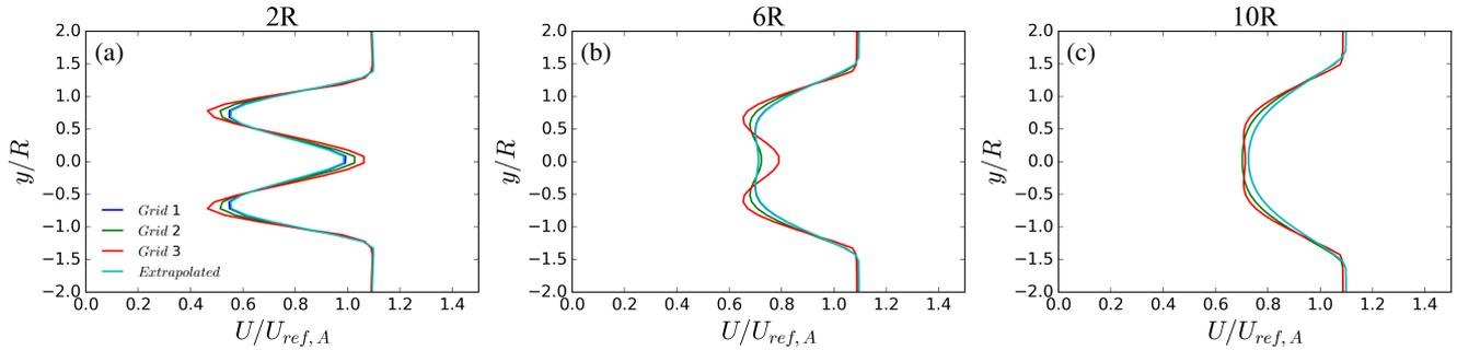
**Figure 2.** Normalised axial velocity computed behind a single model wind turbine (case A) for three grids at (a)  $x/R=2$ , (b)  $x/R=6$  and (c)  $x/R=10$  for the  $k-\varepsilon$  turbulence model and the polynomial distribution.
