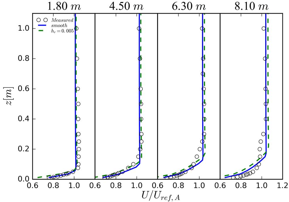
**Figure 3.** Axial velocity for different wall functions plotted against the experimental data for four downstream distances from the inlet.
