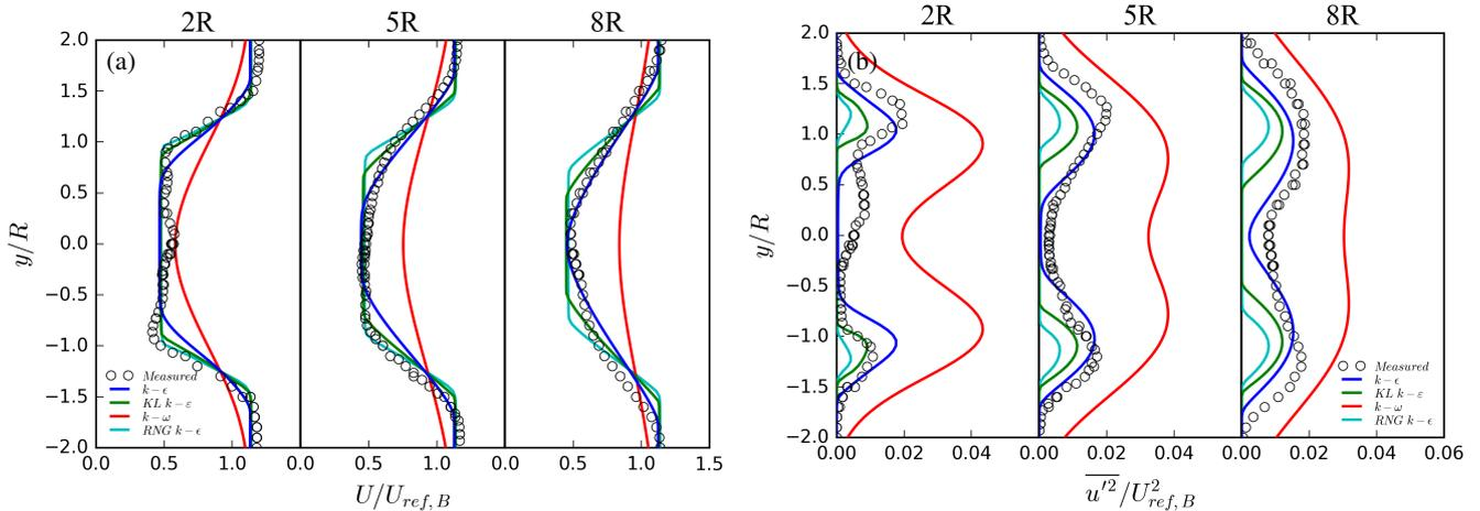
**Figure 7.** (a) Normalised axial velocity and (b) normalised stream-wise variance of the velocity computed for the two in-line model wind turbines (case B) at  $x/R = 2, 5$  and  $8$  downstream of the second wind turbine for different turbulence models using the undistributed thrust.
