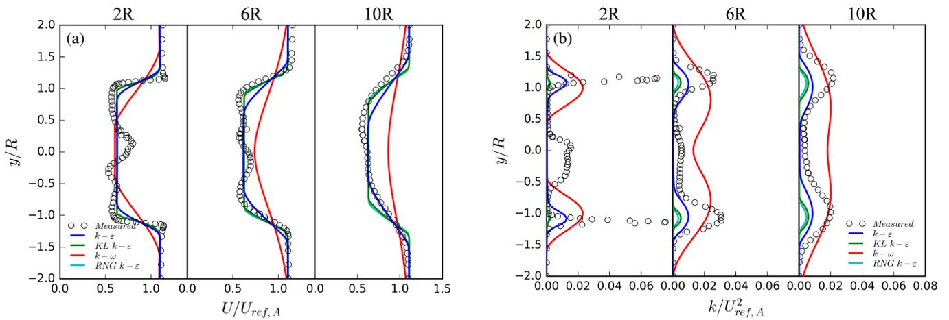
**Figure 5.** (a) Normalised axial velocity and (b) normalised turbulent kinetic energy computed behind a single model wind turbine (case A) at  $x/R = 2, 6$  and  $10$  for different turbulence models using the uniform distribution.
