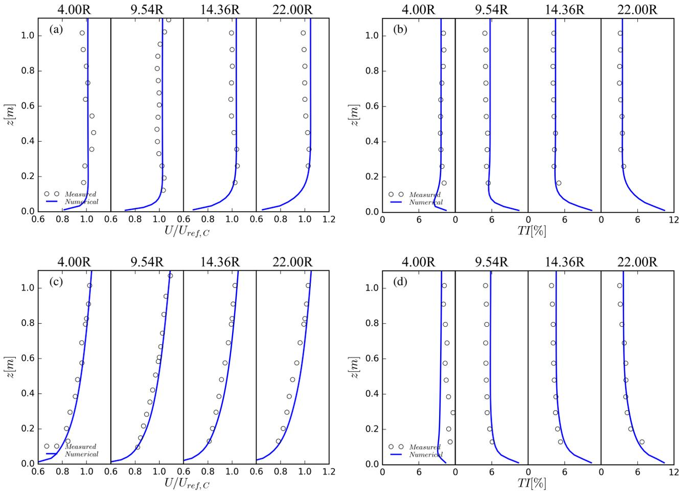
**Figure 9.** Empty domain stream-wise velocity and turbulence intensity results for Case C1 (a),(b) and Case C2 (c),(d) for four vertical profiles downstream of the inlet when using the  $k - \varepsilon$  turbulence model.
