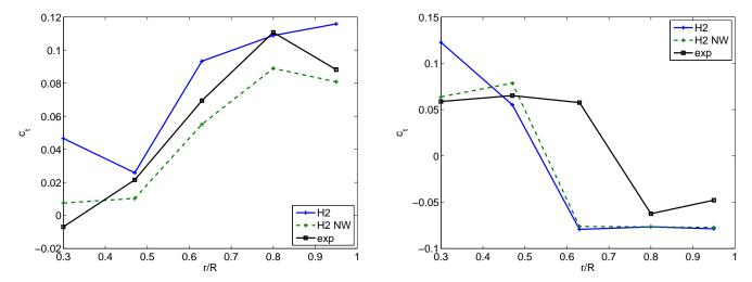
**Figure 5.** Radial distribution of tangential force coefficients at 3.5 (left) and 18.2 (right) degrees geometric AOA at 47% blade radius. Results from HAWC2 (denoted H2) and HAWC2 including the extended near wake model presented in this paper (H2 NW) are compared to measurements.
