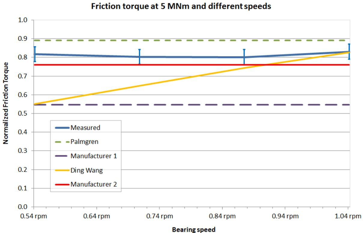
**Figure 9: Measured and calculated friction torque at different speeds and 5 MNm load**
