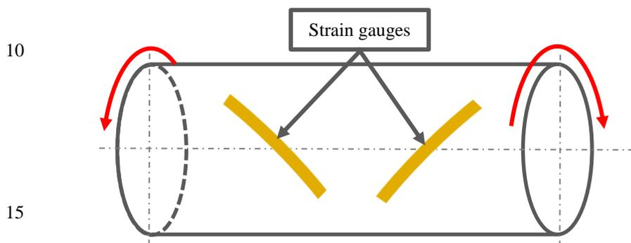
Figure 3: Torque measurement strain gauges on shaft.
