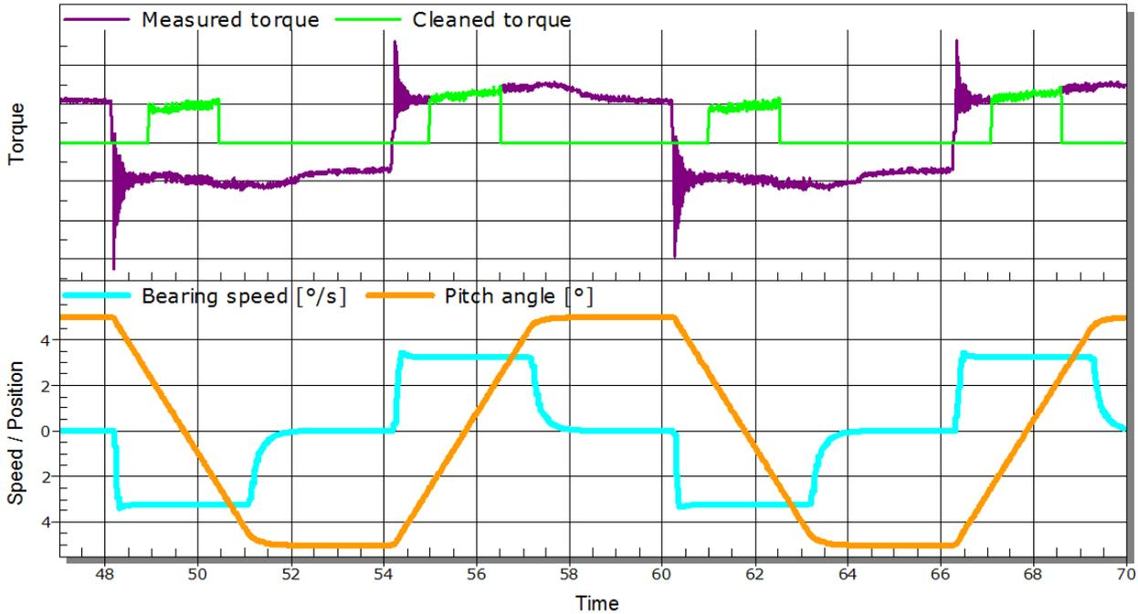
**Figure 4: Oscillating rotations and torque measurements (example)**
