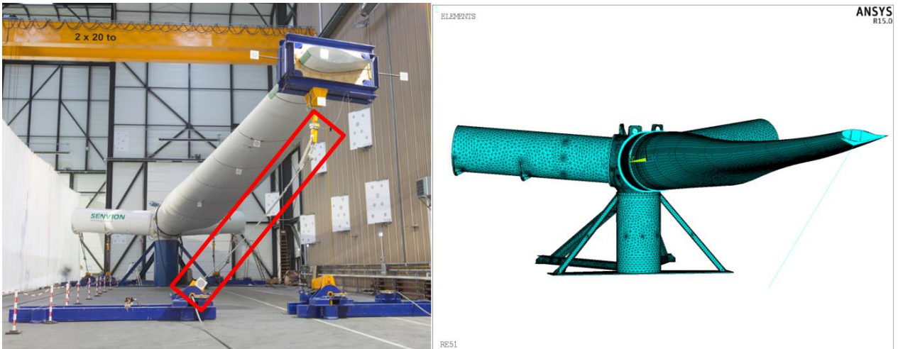
Figure 1: Pitch bearing test rig at Fraunhofer IWES and corresponding FE model.
