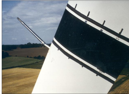
Figure 1. Five-hole pitot tube mounted at the blade of a 95kW Tellus turbine at Risø in 1995
