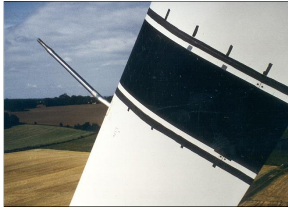
Figure 1. Five-hole pitot tube mounted on the blade of a 95kW Tellus turbine at Risø in 1995
