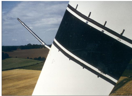
Figure 1. Five-hole pitot tube mounted on the blade of a 95kW Tellus turbine at Risø in 1995
