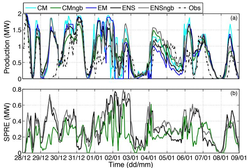
**Figure 11.** a) Production forecast in MW at site A for the different approaches (Figure 3). For CMngb, ENSngb and ENS the lines present the average of the multiple forecasts. Observed production is given with the dash-dotted line. The production is calculated for a 2 MW-turbine. b) The spread of the multiple members in CMngb, ENSngb and ENS.
