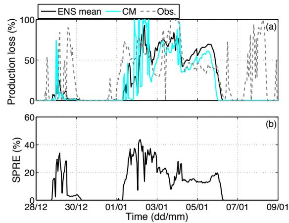
**Figure 7.** Site A. a) Forecasted production loss in percent. Black line is the ensemble mean using ENS, green line is the CM and dashed grey line is the observed production loss. b) The related spread of the ensemble members in ENS.
