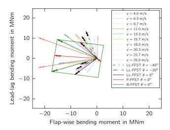
**Figure 5.** Moment vectors of lead-lag loading at different wind speed bins and in a lead-lag fatigue full-scale blade test (**FFSTLL-FFST**) at different pitch angles at 10 % blade length. A flap-wise FFST (F-FFST) and the bounding box of possible bi-axial FFST scenarios (B-FFST) is shown.
