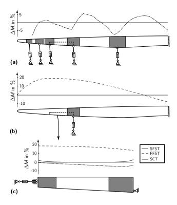
Figure 1. Load deviation  $\Delta M$  between test bending moment and target bending moment determined for the DTU10MW blade and test setup for static full-scale test (SFST) in side view (excerpt from Antoniou et al. (2015)) (a), fatigue full-scale test (FFST) in top view (b), and blade cut-out sub-component test (SCT) (c). Untested areas are shown in gray.
