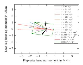
**Figure 6.** Moment vectors of lead-lag loading at different wind speed bins and in a lead-lag fatigue full-scale blade test (**FFSTLL-FFST**) at different pitch angles at 70 % blade length. A flap-wise FFST (F-FFST) and the bounding box of possible bi-axial FFST scenarios (B-FFST) is shown.
