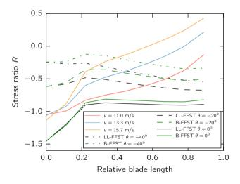
**Figure 8.** Stress ratio *R* of the axial strain along the trailing edge bond line at different wind speed bins, and lead-lag (LL-FFST) and bi-axial (B-FFST) fatigue full-scale blade tests (FFST) at different pitch angles.
