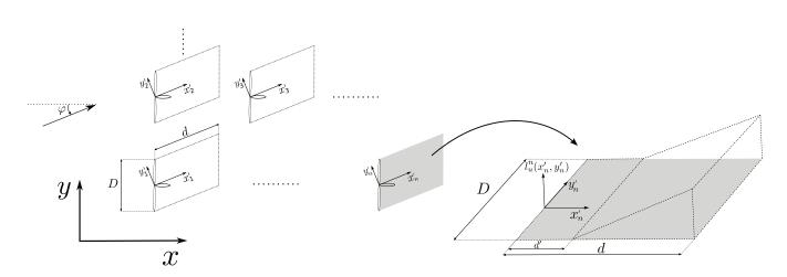
Figure 3. Schematic illustration of the mixing length.
