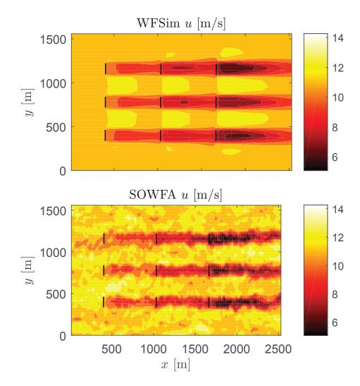
Figure 16. Flow field obtained with SOWFA (below) and WFSim at t = 250 [s]. The black lines indicate the turbines.
