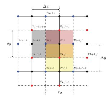
**Figure 5.** One cell for the x-momentum equation (grey with in its centre  $u_{i,J}$ ), one for the y-momentum equation (yellow with in its centre  $v_{I,j}$ ) and one for the continuity equation (pink with in its centre  $p_{I,J}$ ). All three cells have equal dimensions and overlap.
