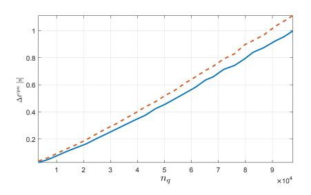
Figure 7. Mean computation time per simulation time step  $\Delta t^{cpu}$  versus number of states  $n_q$ . Red dashed is WFSim as presented in (20) and blue is WFSim as presented in (21). Note that the number of cells is approximately  $n_q/3$  with  $n_q$  the number of states.
