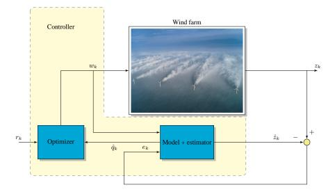
Figure 1. General dynamic closed-loop dynamic control framework with measurements  $z_k$  and its estimation  $\hat{z}_k$  and state estimation  $\hat{q}_k$ . The signals  $r_k$  and  $w_k$  are a reference and control signal, respectively. In this paper we present a dynamic model that is compatible with this framework.
