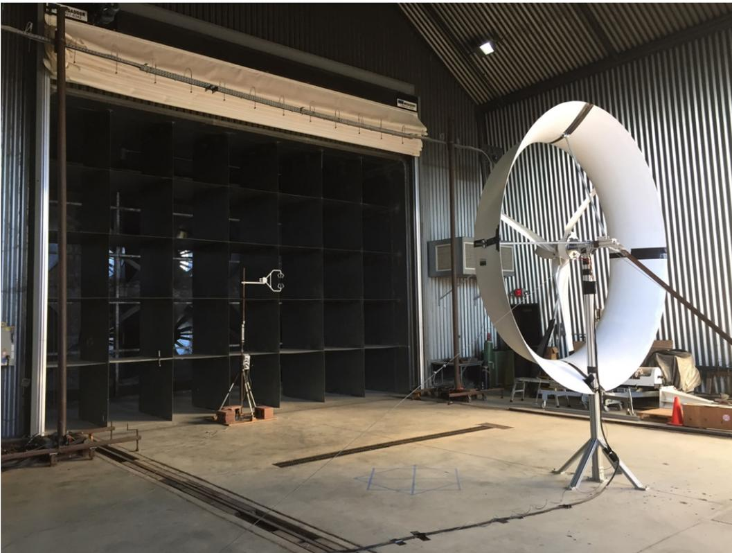
**Figure 12: Ducted Rotor Under Test Conditions.**
