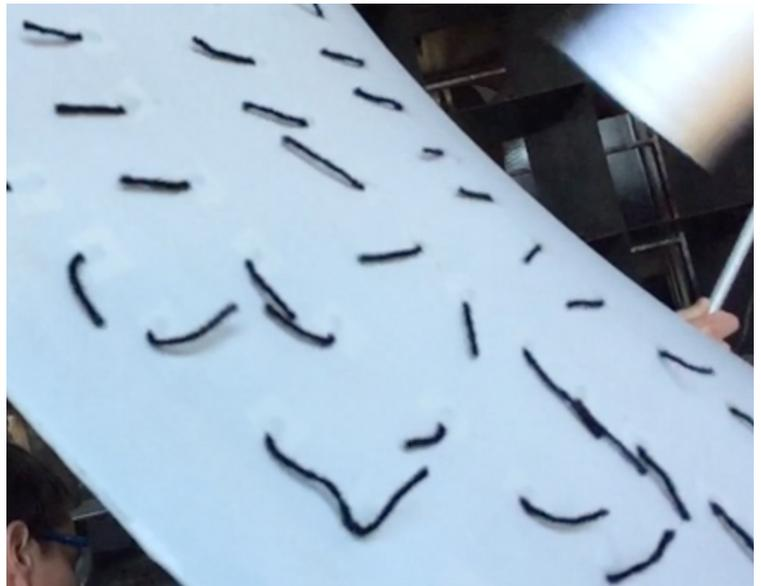
**Figure 15: Tufting on the Ducted Surface.**
